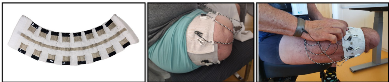
Fig. 1 Textrode-band (left) and participants wearing the Textrode-band (middle and right): the middle panel demonstrates application on a shorter residual limb, whereas the right panel illustrates usage on a longer residual limb
