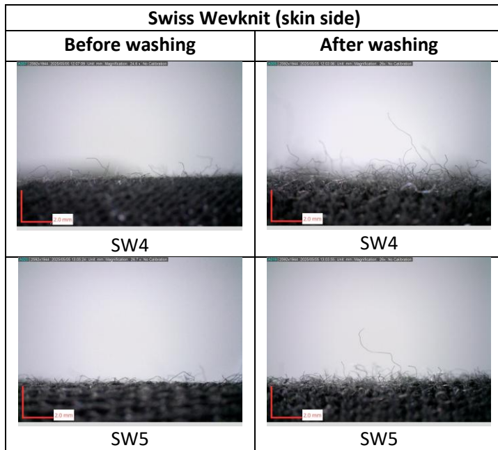
Figure 12. Fabric surface of Swiss wevknit before and after washing
