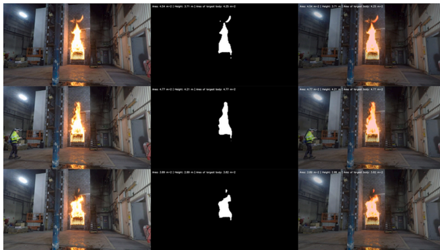
Fig. 2. The figure depicts three distinct time points during the fire test, where a prediction is generated by U-Net. The predicted segmentation mask is presented in binary form in the center and is subsequently overlaid on the original image to the right.
