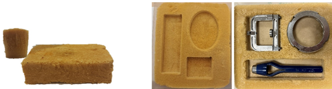
FIGURE 4 | MBF that are molded in cylinder and cubic and its prototype as cushioning packaging.
