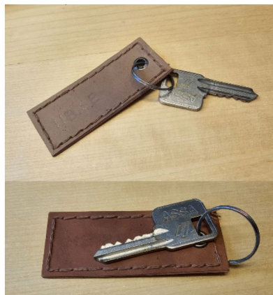
Fig. 9. The prototype made using Chestnut (Chestnut C GB-top picture) and Indusol ATO (Indusol ATO C GB-bottom picture) composites after glycerol and bio-based binder post-treatments (on either sides).
