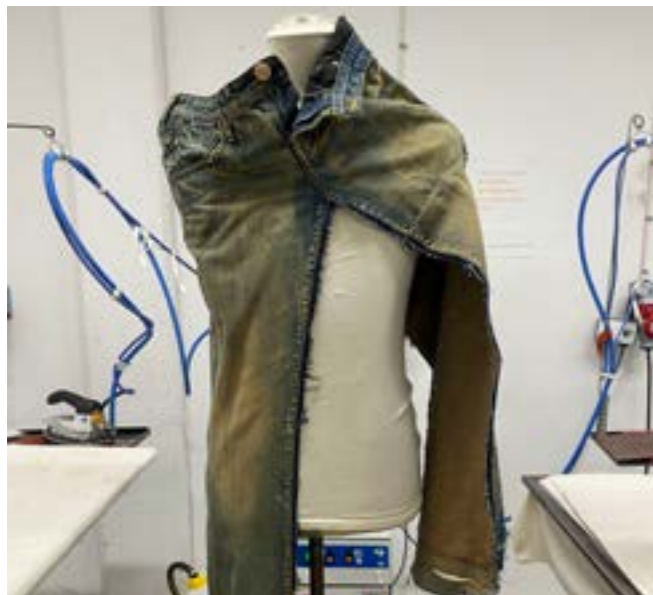
Figure: 94. Fig 92-95. Showing how garments have been further developed through out the process. The blu elasthan jacket has been replaced with a thicker RAW denim material and there are also a change of dye.
