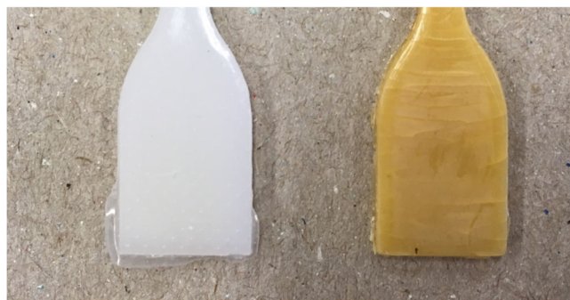
FIGURE 1 Test body before aging (left) and after 10 weeks of aging (right) [Color figure can be viewed at wileyonlinelibrary.com ]
