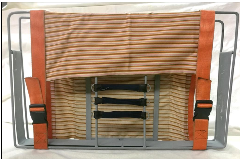
Figure 28. Picture of fire hose basket
