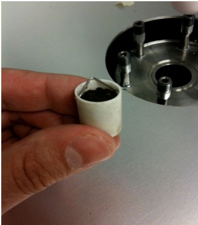
Figure 11. Powdered black residue after Treatment
