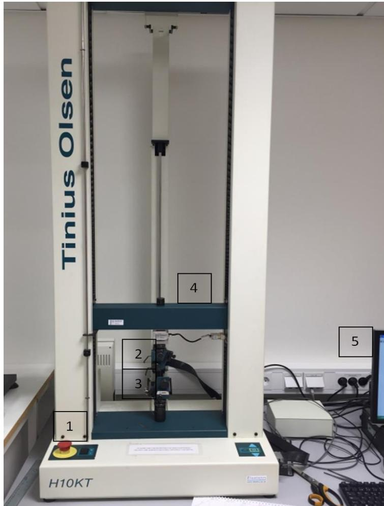
Figure 17- Tensile testing for composite with equipment's: 1-Power button; 2-Upper jaw; 3-Lower jaw; 4-Crosshead; 5-Computer display
