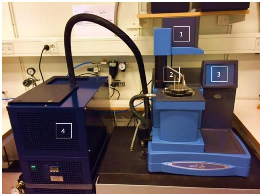
Figure 19- Experimental DMTA equipment with instruments mentioned in square box: 1- Furnace; 2- Dual cantilever clamp; 3- Display; 4- Cooling chamber with liquid nitrogen gas
