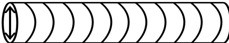
Figure 28- Circular weft knitting has large expanding stiffness due to its extensibility
