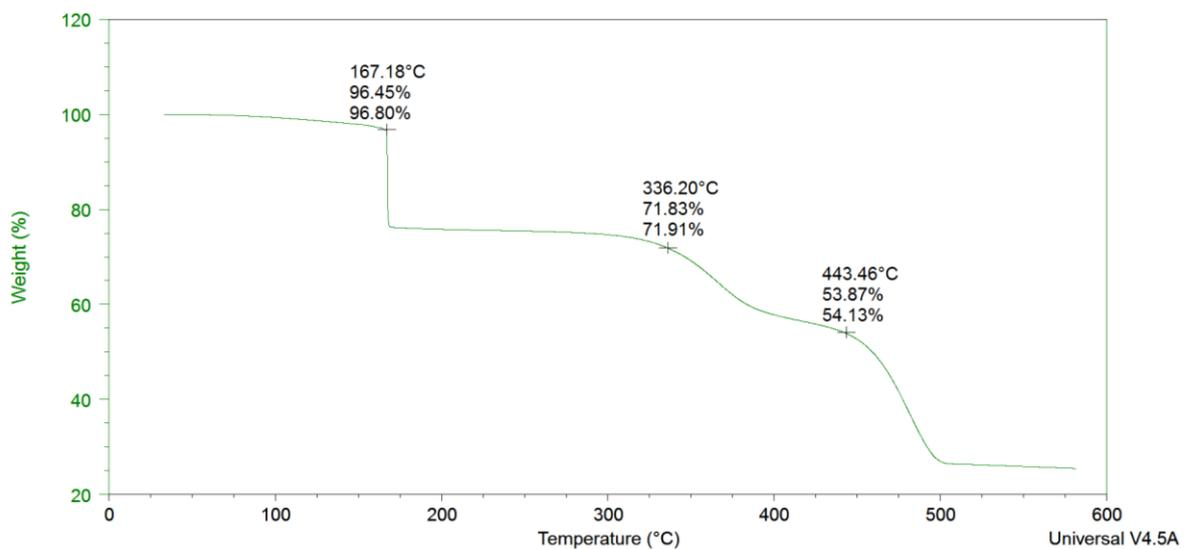
Figure 26 Representative of a drop in Tg at 167°C and later in two stages at 336°C and 443°C
