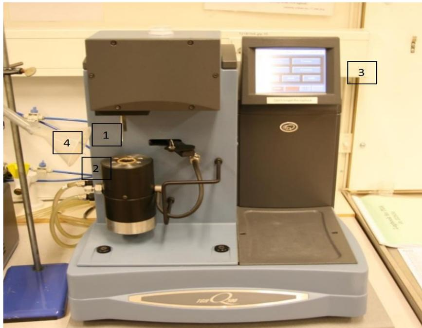
Figure 21-TGA instrument with equipment's: 1- Specimen vessel; 2- Specimen chamber; 3- Display; 4-Air passed to cool the vessel.
