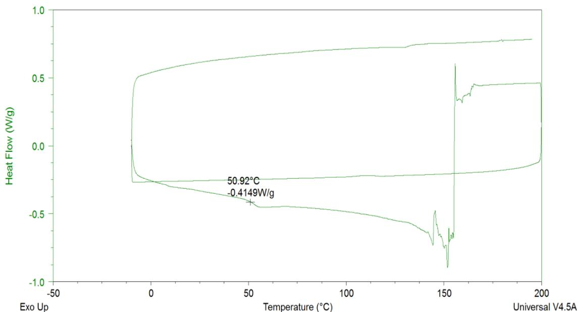
Figure 24 Representative of a drop in T<sub>g</sub> at 50.92°C and further Dyneema melts around 145°C
