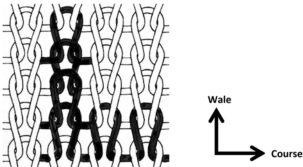
Figure 4 Knitting structure showing knitting direction in wale and course direction
