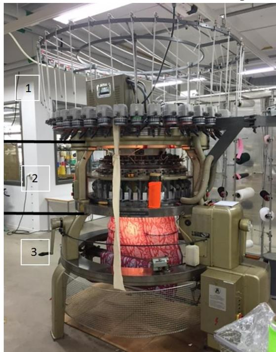
Figure 10- Double jersey weft knitted fabric using rib structure: 1-Creel system; 2-Knitting system; 3-Fabric take down system
