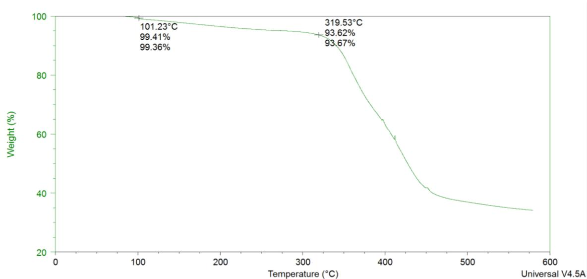
Figure 27- Representative of a drop in Tg at 101°C and 319°C
