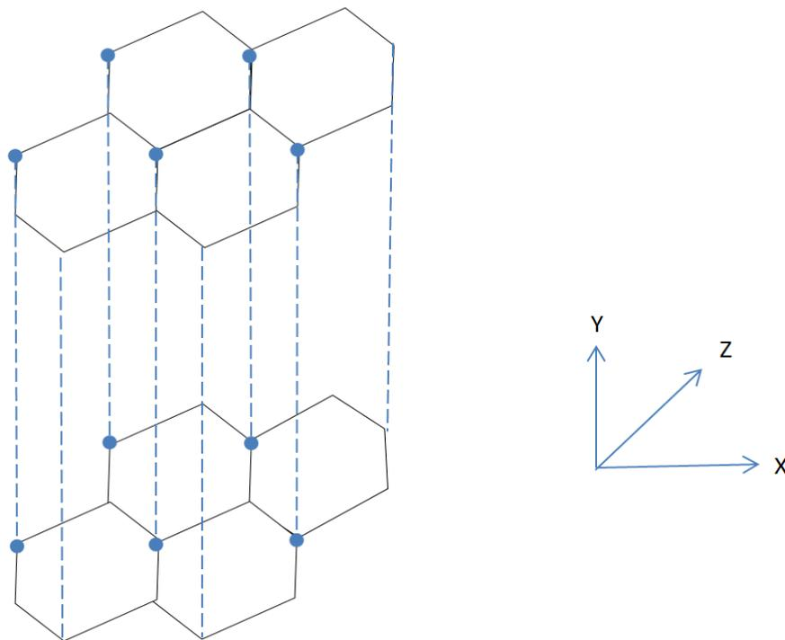
Figure 3 Crystal structure of the carbon fiber
