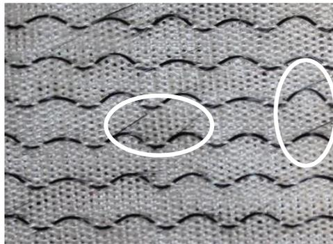
Figure 14 Single jersey knitted fabric on every 4<sup>th</sup> needle and circle showing breakage of carbon fibers
