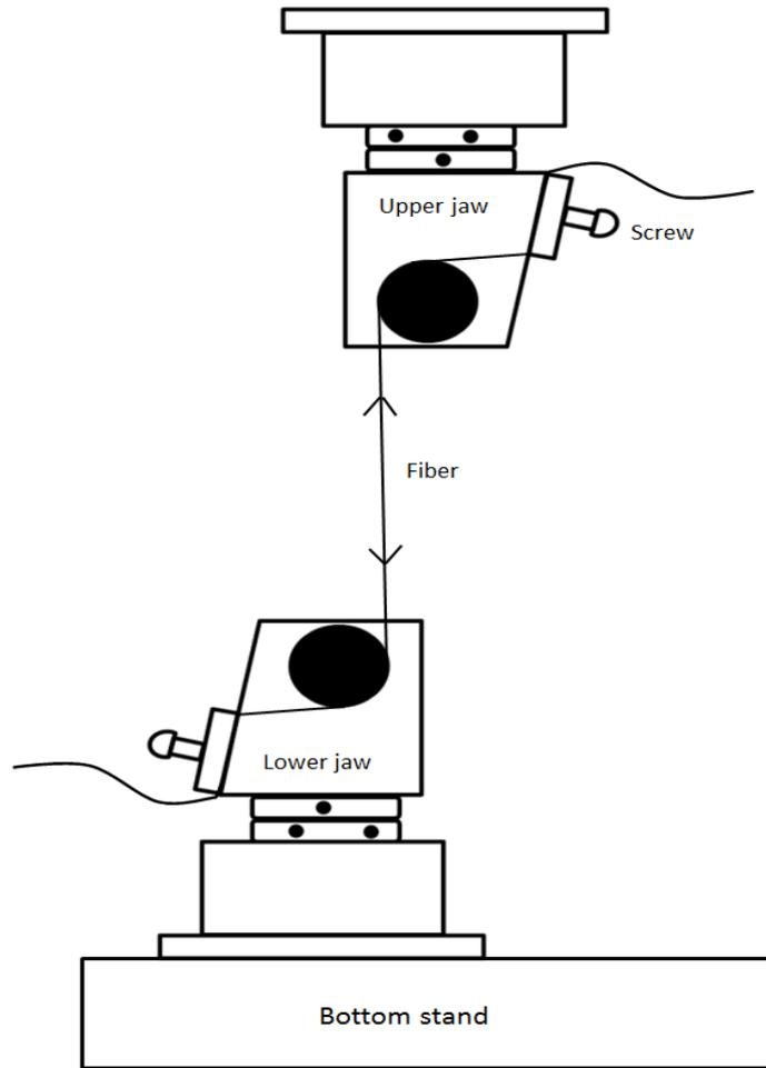
Figure 13 Tensile testing instrument with equipment's mentioned
