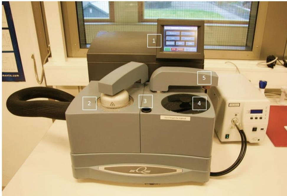
Figure 20- DSC instrument with equipment's: 1-Display; 2-Specimen chamber; 3-Used pan bin; 4-Pans placement chamber; 5- Robotic pan mover.
