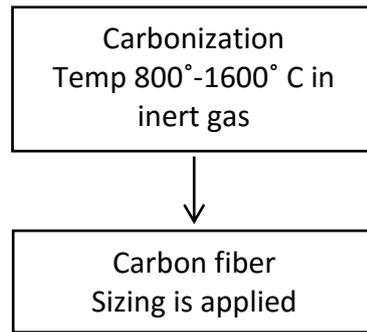
Flowchart 1 Carbon fiber manufacturing process
