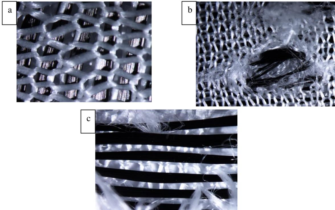
Figure 16 Microscopic test for knitted fabric a) Normal knitted fabric from the top view b) Surface/Dyneema® fibres were removed slowly without disturbing the carbon fibres c) Zoomed in for the carbon fibres.
