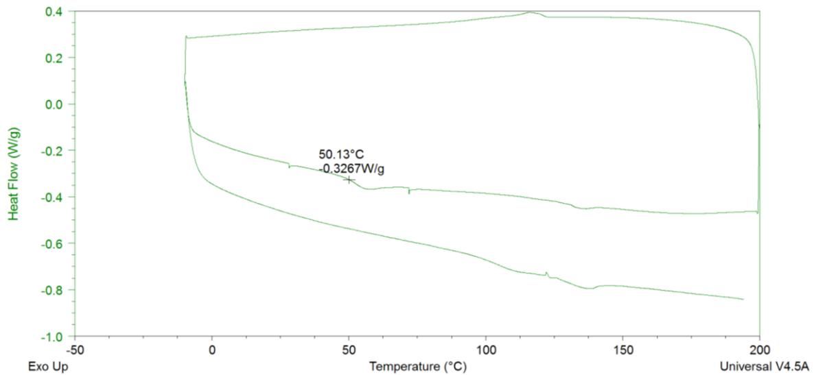
Figure 25 Representative of a drop in Tg at 50.13°C and further polyester melts around 120°C
