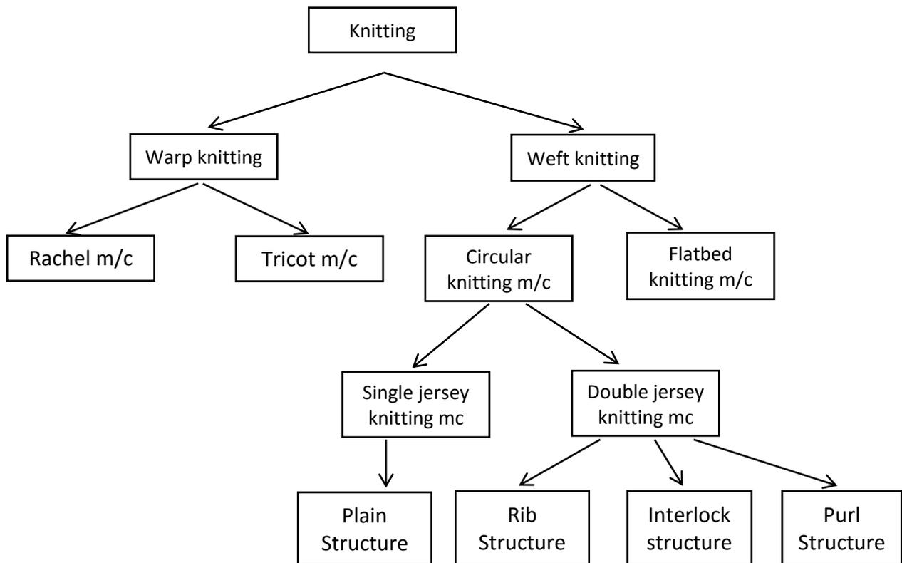
Flowchart 2 Classification of knitting based on knitting types, knitting machine and knitting structures
