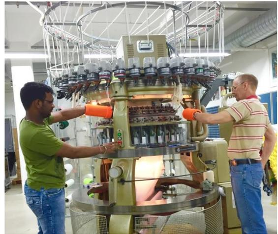
Figure 9 Carbon bobbins are hold in hand to pass the yarns straight to feeder
