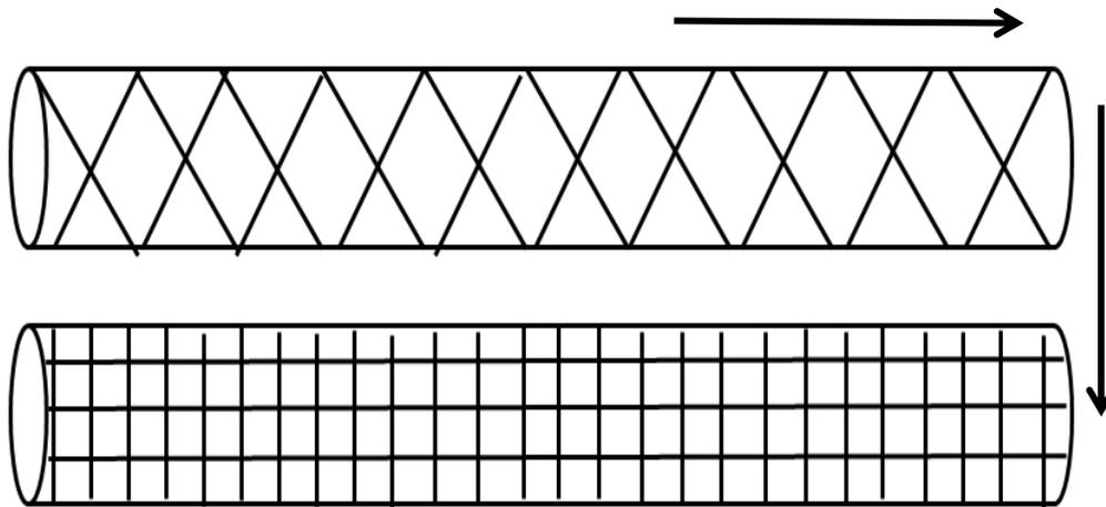
Figure 27- Braiding and weaving has good bending and torsional stiffness
