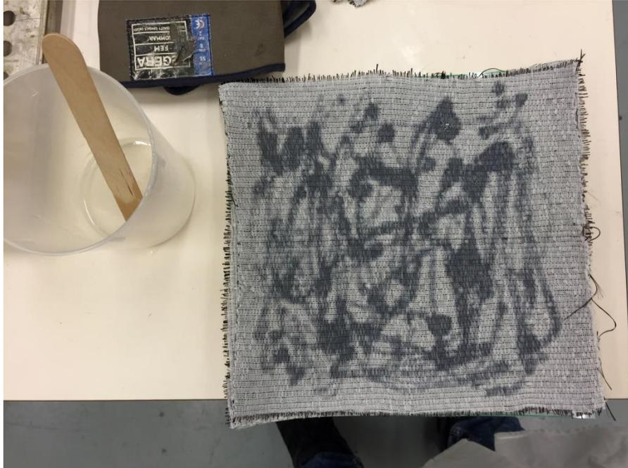
Figure 11 Resin distributed equally on the fabric with a foil beneath
