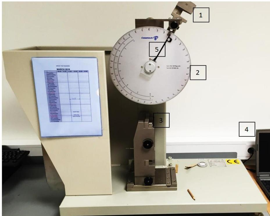
Figure 18- Impact testing instrument with equipment's: 1-5J weight; 2- Impact measuring scale; 3- Specimen mounting place; 4- Computer; 5- Needle.
