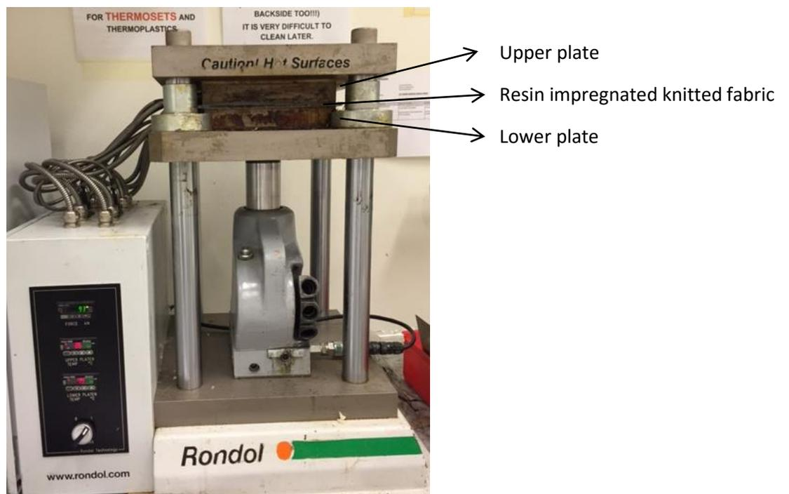
Figure 12 Compression molding machine with digital temperature and applied pressure display
