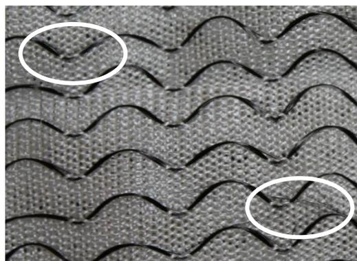
Figure 15 Single jersey knitted fabric on every 8<sup>th</sup> needle and circle showing breakage of carbon fibers
