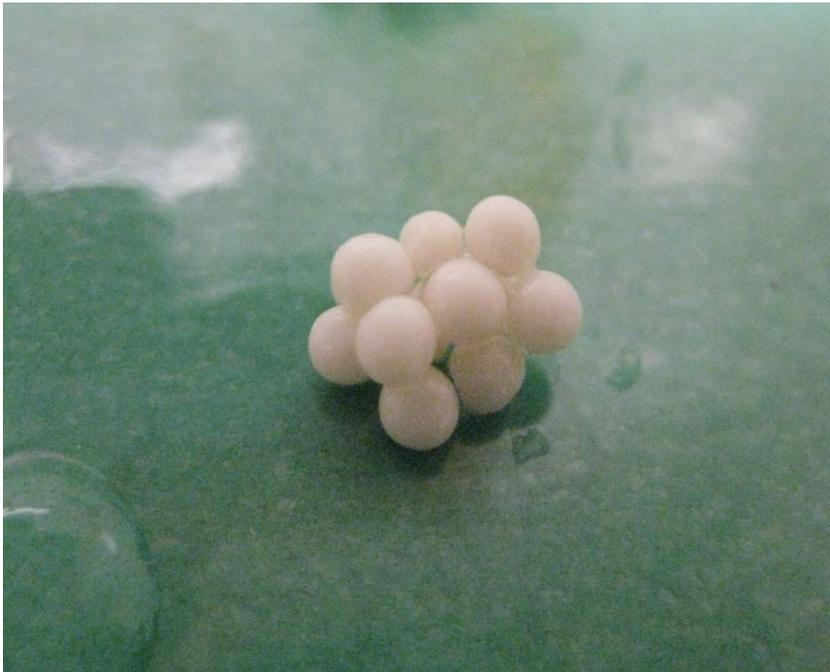
Figure 5 Alginate chitosan capsules with filled yeast biomass
