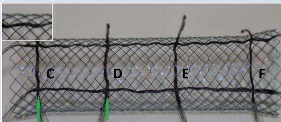
Figure 1 A stent with integrated piezoelectric fibres
