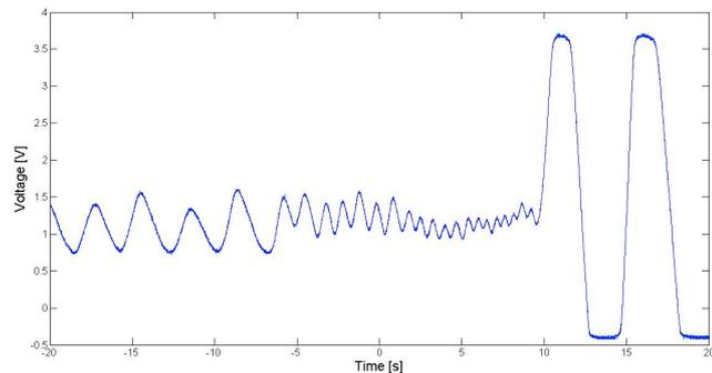
**Figure 1:** Different respiration patters recorded by the developed system. About 15s normal, 15s shallow and 10s of deep breathing.
