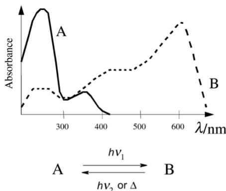
Figure 1: Difference in absorption spectra of colourless state A and coloured state B [5]
