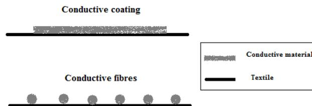
**Figure 4** Difference in coverage on the textile surface.
