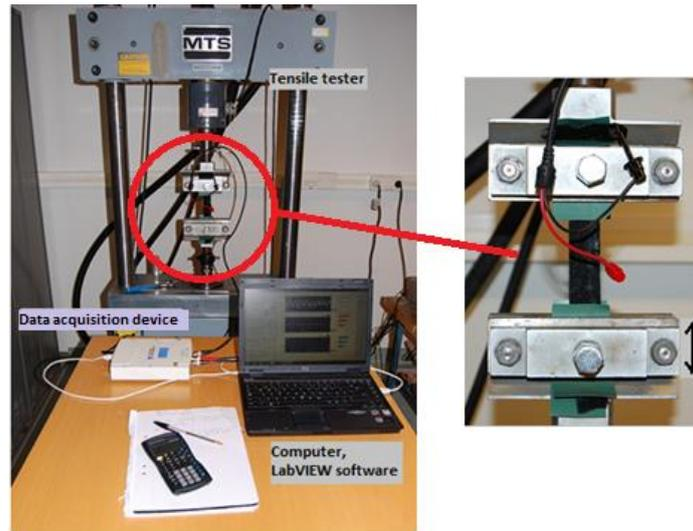
Figure 1 Tensile testing machine set up for characterisation
