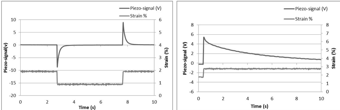
**Figure 3** Coated sample in plain weave (left), Statex fibre in weft in plain weave (right). A pre-load was set to 30 N and a strain of 1 % was applied.
