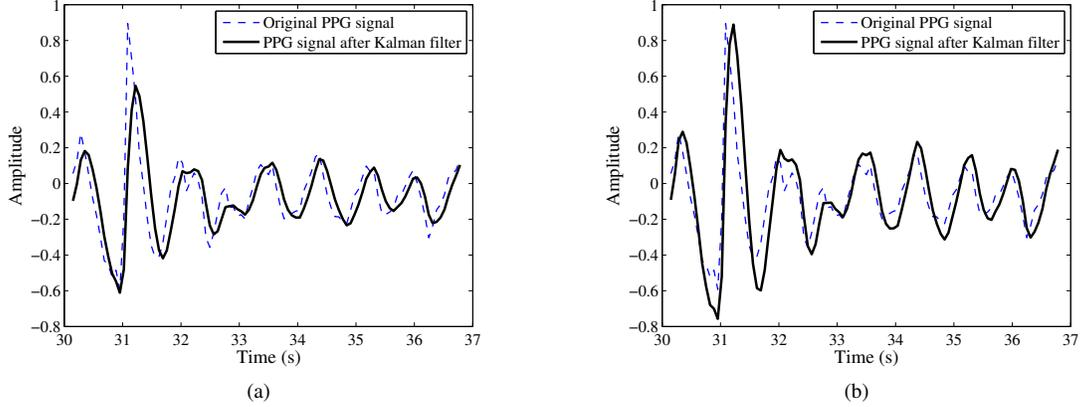
Fig. 2: The comparison of the original PPG signal and that after Kalman filter. In Figure (2a),  $H = [1 \ 0 \ 0]$ , the high-frequency noise in the signal is eliminated and the heart pulse is remained. In Figure (2b),  $H = [0 \ 0 \ 1]$ , the heart pulse is enhanced after filtering.
