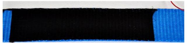
Figure 2. Conductive coated sensor on cargo security straps
