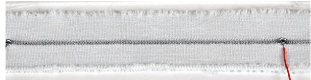
Figure 2: knitted stretchable sensor made by conductive yarn.
