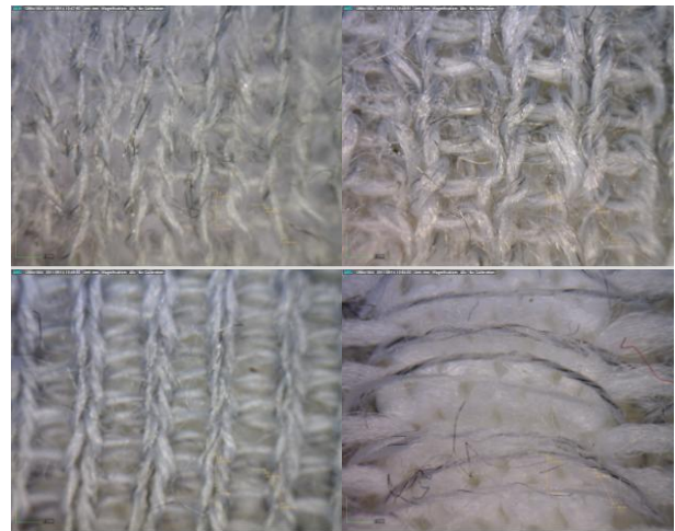
Figure 3: microscope picture of different structures, Plain Jersey (up left); 1x1 rib (up right); Interlock (bottom left) and Floating (bottom right).
