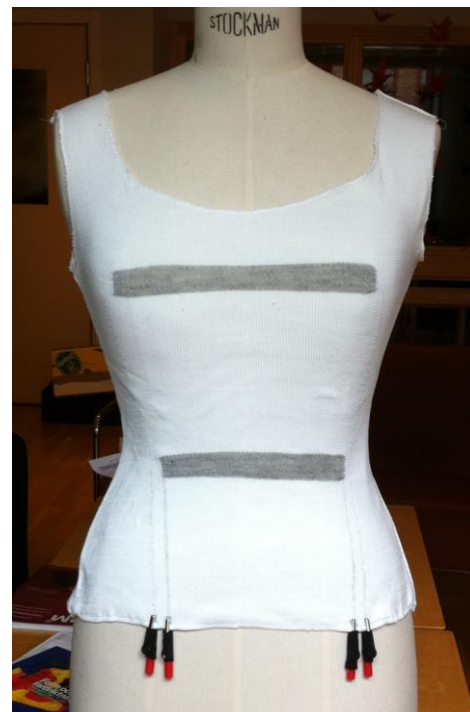
Figure 5. Prototype garment made by flat knitting machine.
