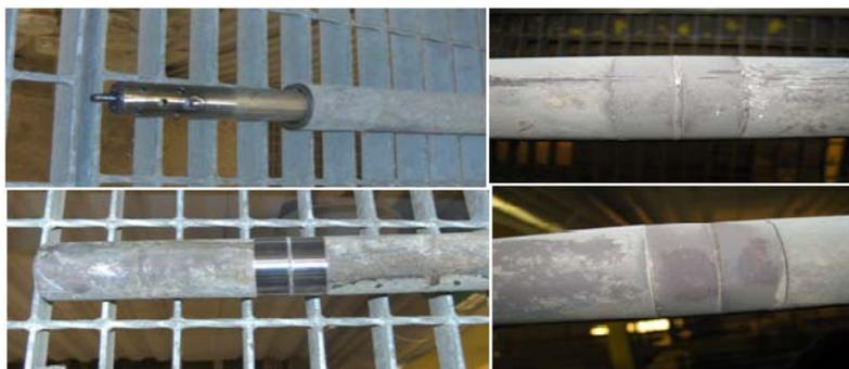
**Figure 2: Deposit probes with sampling rings used in the combustion tests.**
