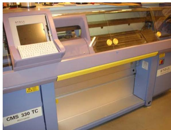
**Figure 2.** The flat knitting machine STOLL CMS 330 TC specially equipped for knitting stiff metallic yarns
