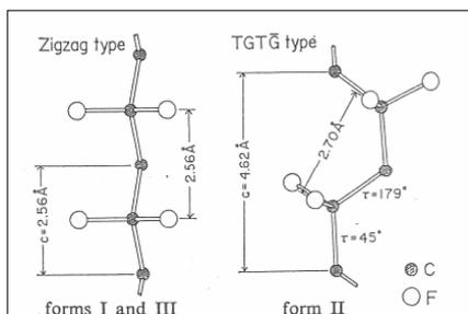
**Figure 1** Molecular structure of the polar  $\beta$ -phase (form I) and the non-polar  $\alpha$ -phase (form II) Reproduced from Ref 1, with permission
