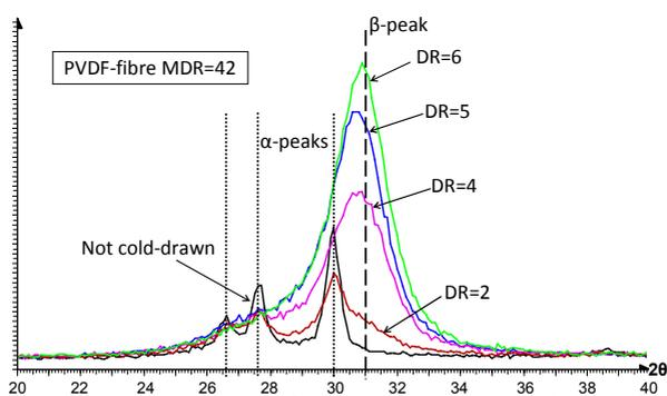
**Figure 2** XRD-patterns for fibres spun at melt draw ratio 42, before and after cold drawing
