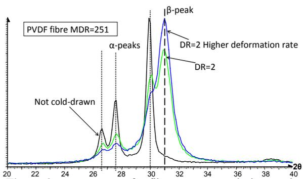
**Figure 3** XRD-patterns for fibres spun at melt draw ratio 251, before and after cold drawing
