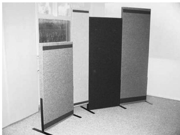
Figure 4. Prototype of an active sound absorbing screen.
