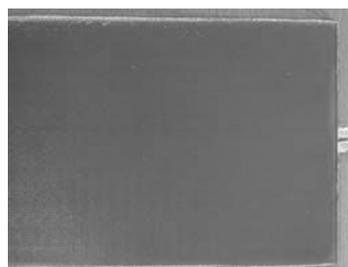
Sample 3: The piezofilm laminated between two layer of woven and heat calendered (350 g/m<sup>2</sup>) polypropylene fabric (11x15 cm).
