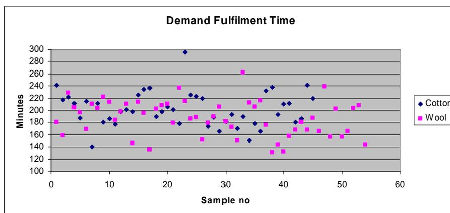
Figure 3: Demand fulfillment time for one 200 hour cycle simulation for own designed garments
