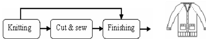
Figure 1: Production process of complete garment concept
