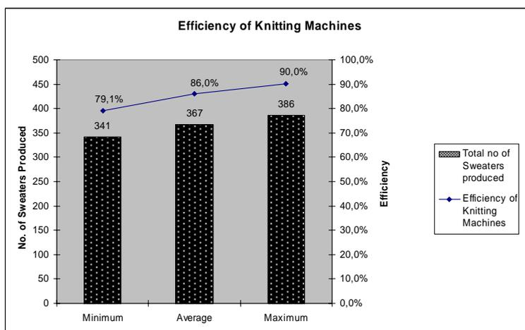
Figure 6: Knitting machines efficiency and total number of produced garments in 15 simulations
