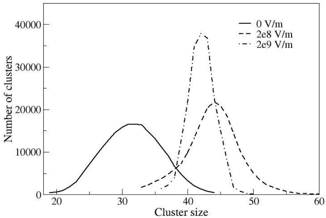
**Figure 11:** Distribution of water cluster sizes in polyethylene systems exposed to different external electric fields at 450 K. The total number of clusters is 200 000 for each system.
