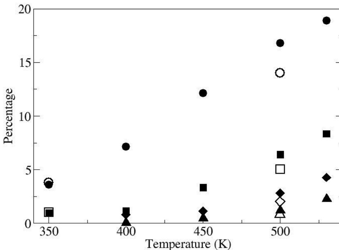
**Figure 6:** Fraction of water molecules included in hydrogen bonded clusters. System size is 200 molecules. Filled symbols are for SPC and open symbols for SPC/E ( only 350 and 500 K ). Dimers ( circles ), trimers ( squares ), tetramers ( diamonds ) and pentamers ( triangles ).
