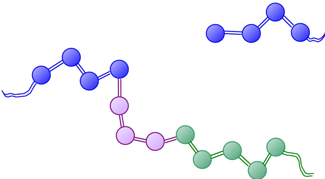
**Figure 9:** End-bridging Monte Carlo. A trimer has successfully been constructed and the left part of the blue chain has been connected to the green chain.
