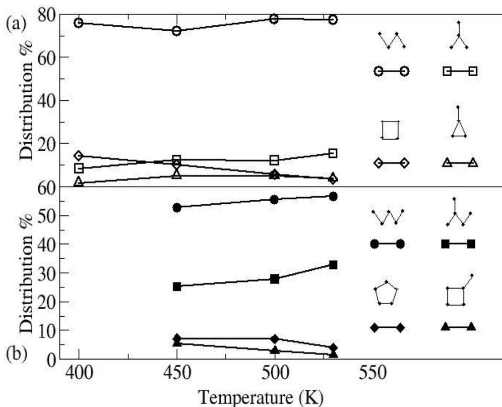
**Figure 7:** Percentage of the four most common SPC tetramer (a) and pentamer (b) topologies between 400 and 530 K.
