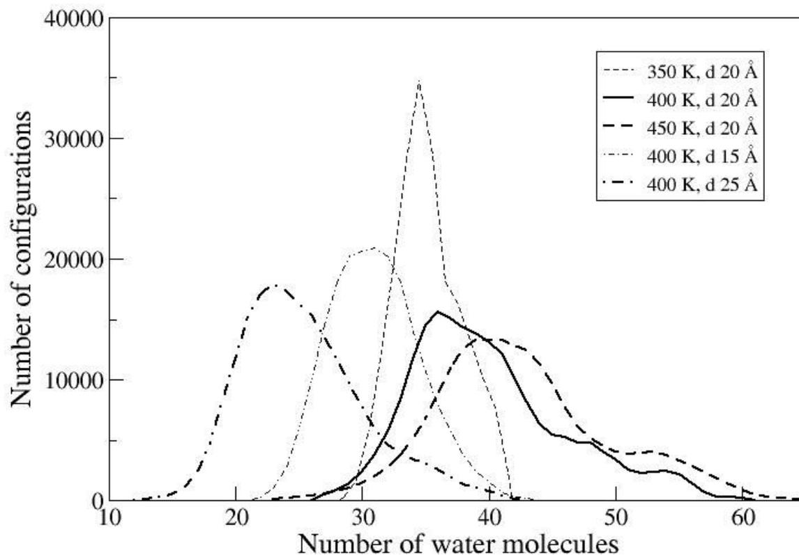
**Figure 10:** Distribution of configurations containing a given number of water molecules in decane, as a function of temperature and Na<sup>+</sup>--Cl<sup>-</sup> distance. The total number of configurations is 200 000.
