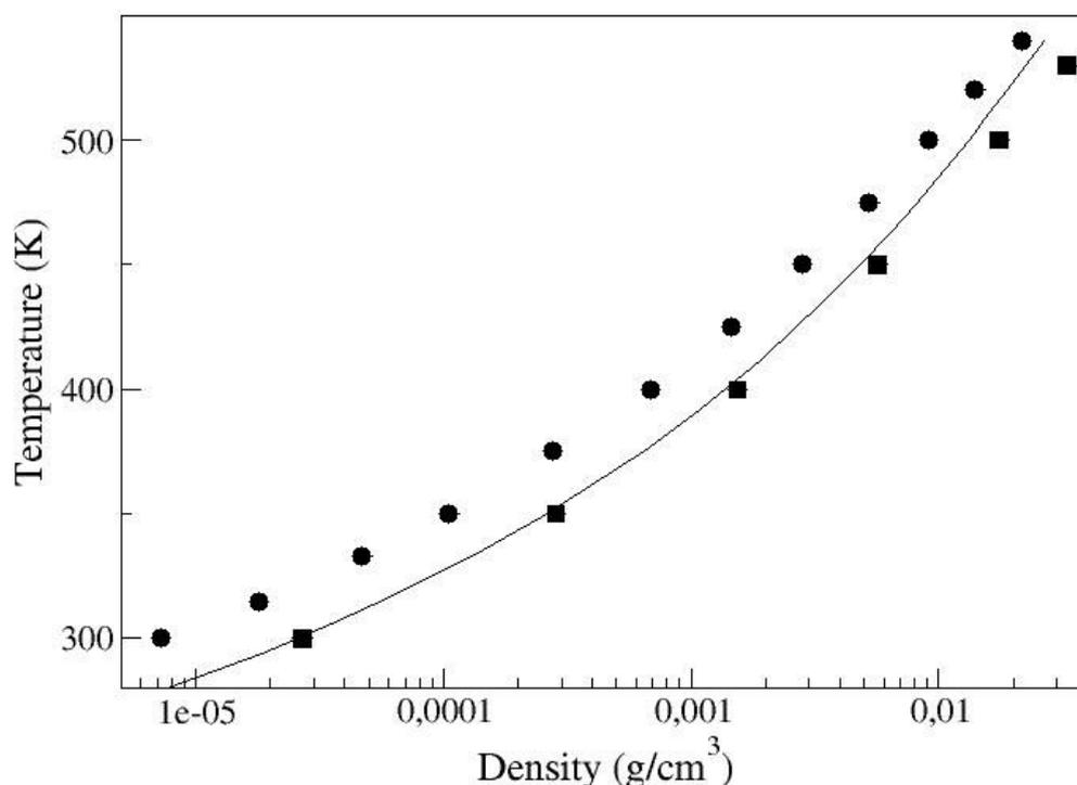
**Figure 4:** Water vapour densities. Data are shown for SPC/E, 500 molecule system, ( circles ) and SPC ( squares ). The solid line shows experimental data. Error bars for both models are much smaller than the symbols.
