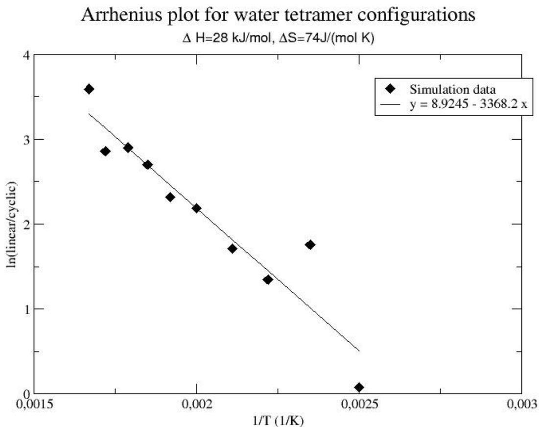
**Figure 3:** Plot of  $\ln(\text{fraction linear clusters} / \text{fraction cyclic clusters})$  vs.  $\text{temperature}^{-1}$ .
