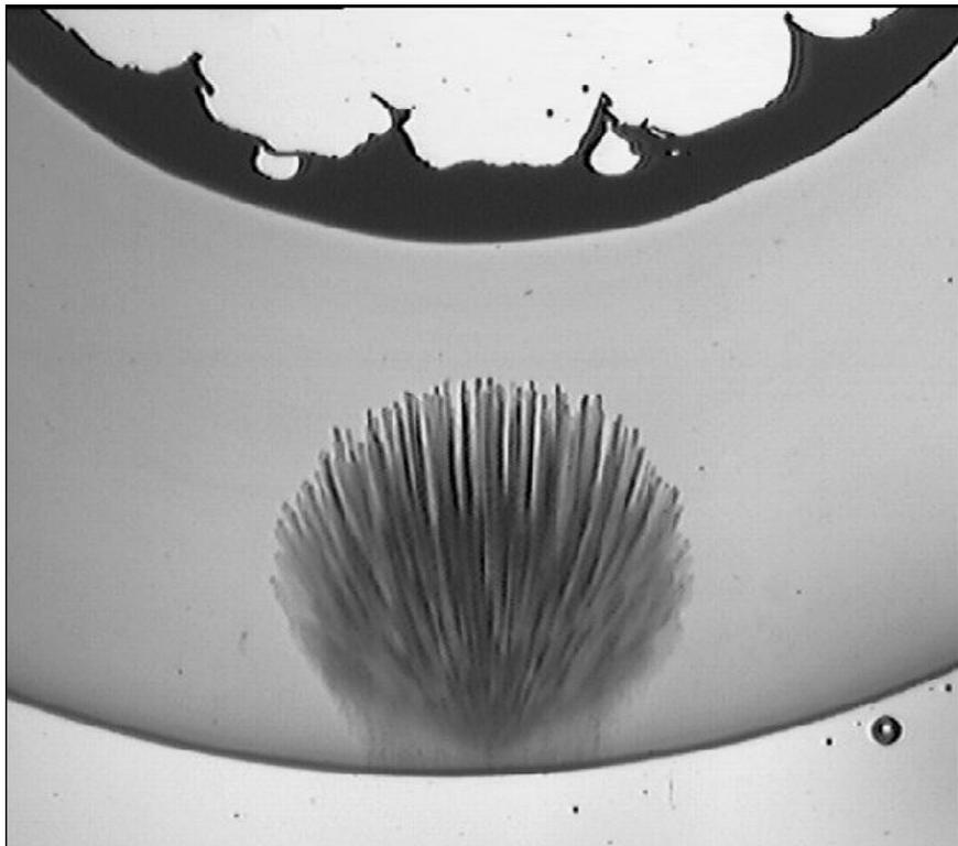
**Figure 1:** Water trees can be seen as tree- or bush-like structures built up by paths of small water containing voids, or in more severe cases, channels in the polymer.
