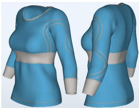
Fig 1: T-shirt for objective monitoring, the gray parts of the garment are the active sensor area. In the early prototypes the sensors are out of traditional electronics, such as accelerometers, commonly used [1] for motion sensing.
