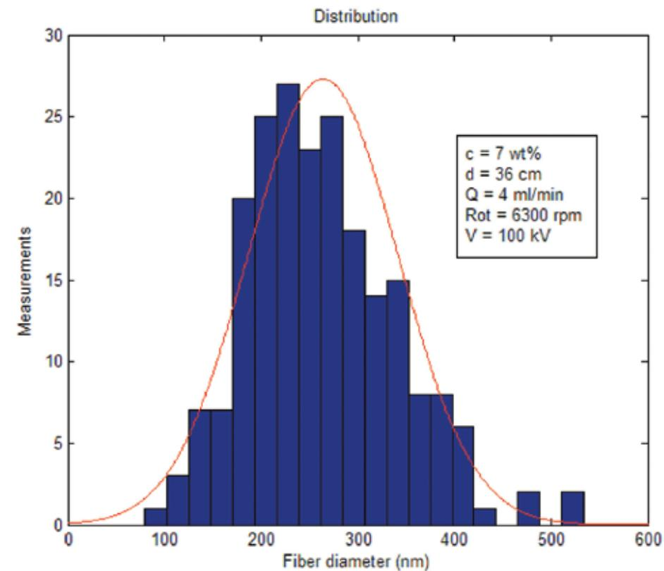
Figure 3. Diameter distribution for over 200 fibers showing a normal distribution
