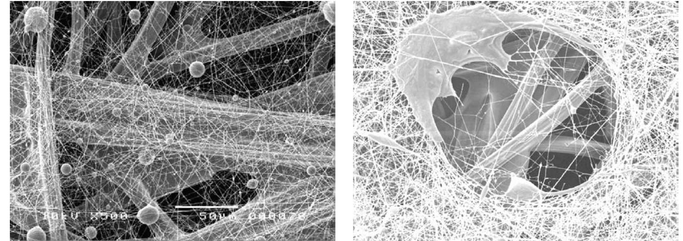
Figure 3. Defects in nanofiber coatings: beads (left) and holes (right). The background seen is the spun bond PET substrate.
