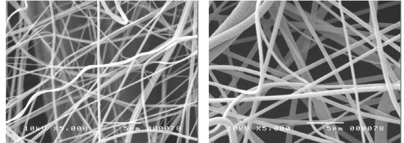
Figure 4. SEM-images (magnification was 5000x at 10 kV) from samples with 10 wt%, 2500 rpm (left) and 16 wt%, 7500 rpm (right). Distance, flow rate and voltage were held constant ( $d=36$  cm,  $Q=4$  ml/min,  $V=100$  kV). The length of the scale bar is 5  $\mu$ m.
