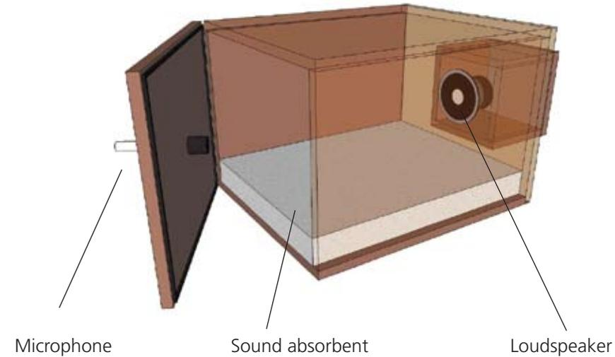
Figure 2. Analysis equipment constructed for quick and cheap qualitative evaluation of sound absorbing properties for thermobonded nonwovens (as shown) and woven fabrics (measured when hanging on a metal rod).
