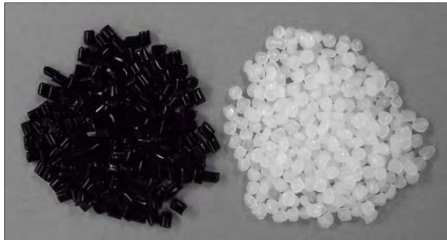
Figure 3. Polymer granules for melt-processing. Right: pure Poly(vinylidene fluoride) (PVDF) supplied from Solvay Solexis. Left: PVDF containing 5 % by weight carbon nanotubes, commercial masterbatch purchased from Hyperion Catalysis, Inc.
