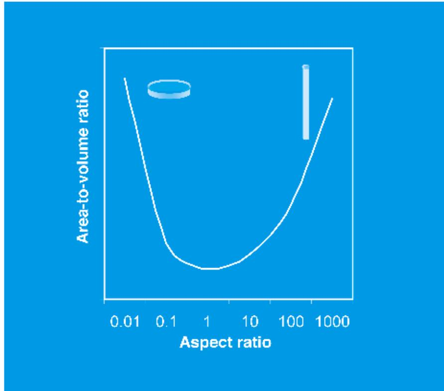
Figure 2. Principle of area-to-volume ratio as function of aspect ratio. (After Gustafsson, 2007)
