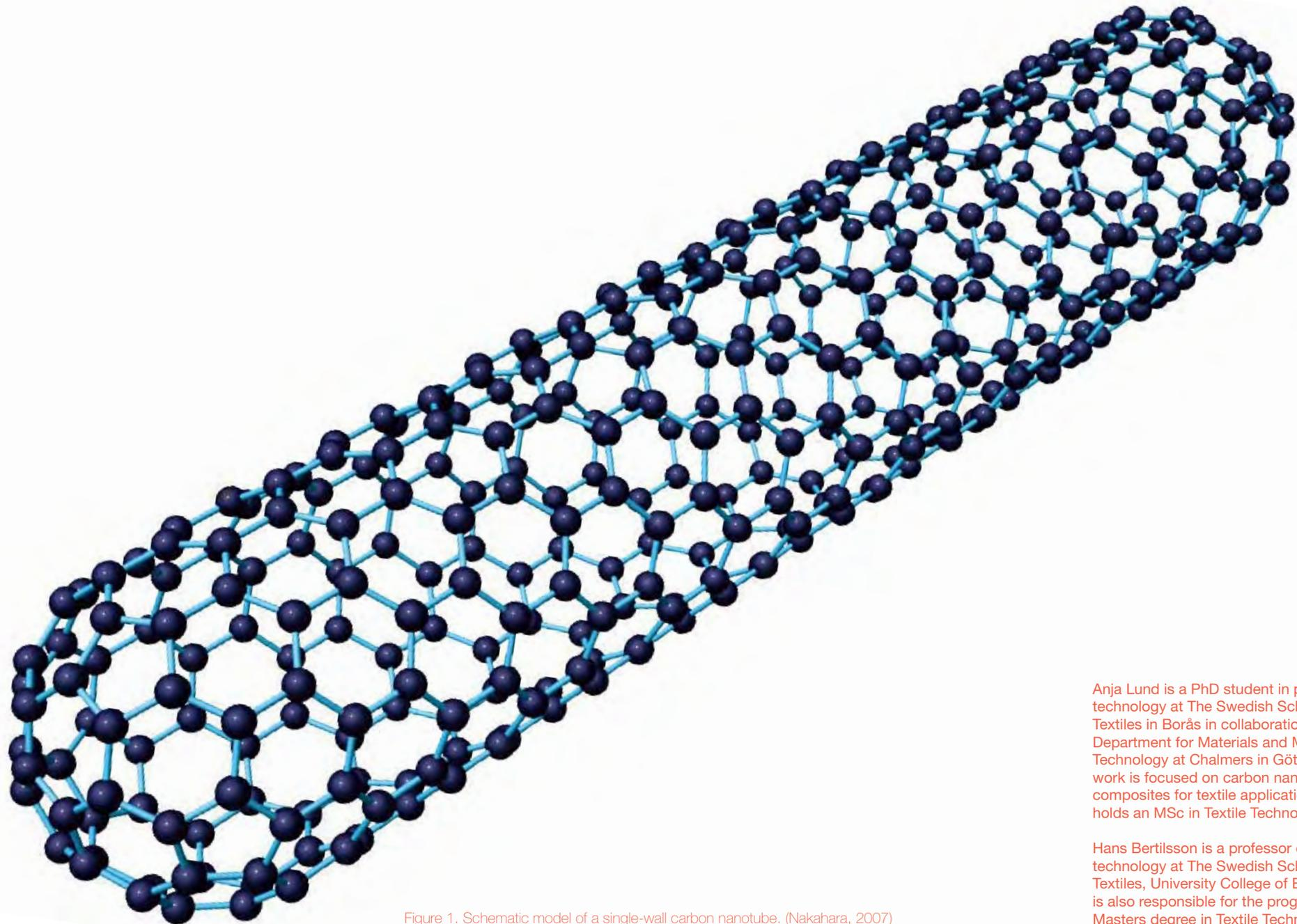
Figure 1. Schematic model of a single-wall carbon nanotube. (Nakahara, 2007)
