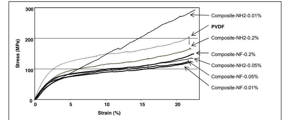
Figure 6. Stress-strain curves for composite fibres prepared by melt-blending and pure PVDF fibre
