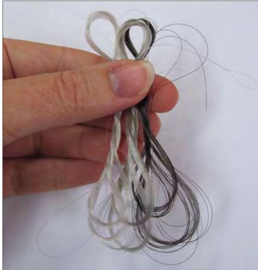
Figure 5. Composite fibres melt-spun from PVDF with varying amounts of carbon nanotubes
