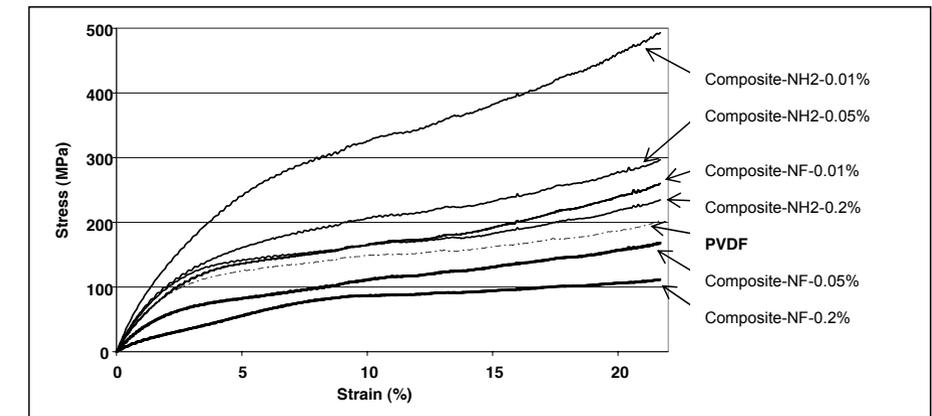
Figure 7. Stress-strain-curves for composite fibres prepared by solvent-aided mixing and pure PVDF fibre (After Gustafsson, 2007)
