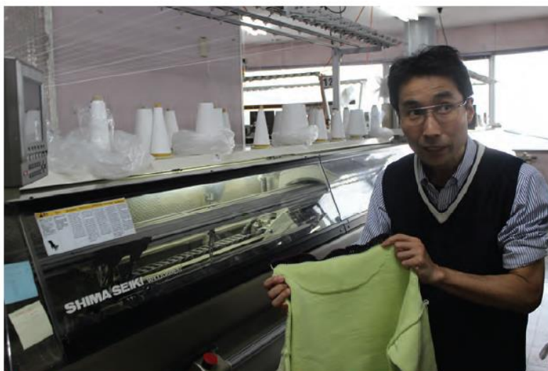
WholeGarment knitwear eliminates the need for cutting and sewing
