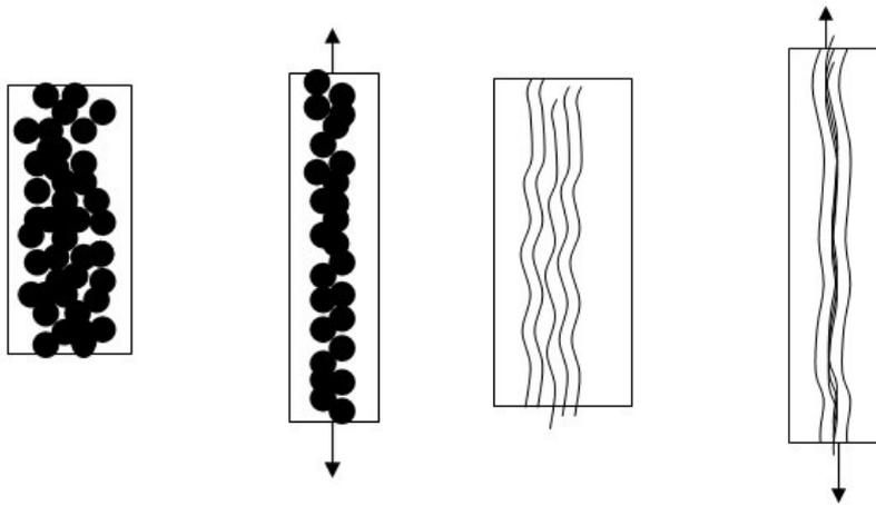
Fig.9. Conductive path of coated sensor (left) and woven sensor (right) before and after stretching.
