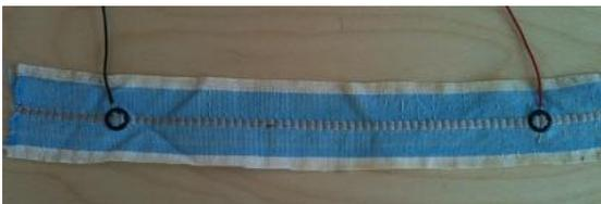
Fig. 5. Inelastic woven sensor, sample 4 (S4)
