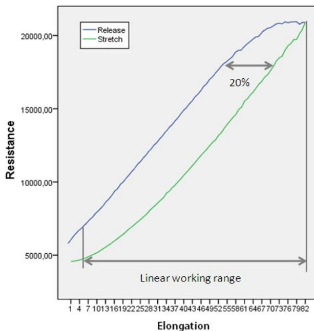
Fig. 11. Hysteresis error of elastic coated sensor, S1
