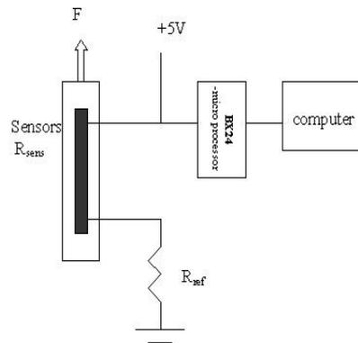
Fig. 7. Electrical measurement setup
