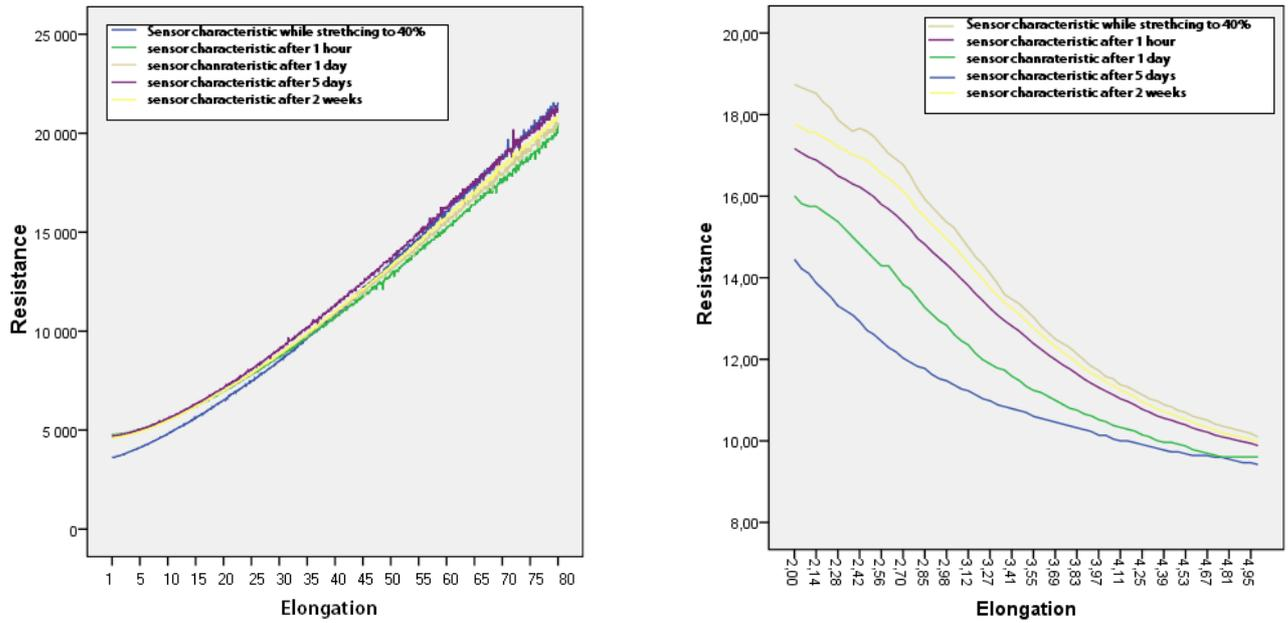
Fig. 10 Stability test during 2 weeks, elastic coated sensor, S1 (top) and inelastic woven sensor, S4 (bottom)
