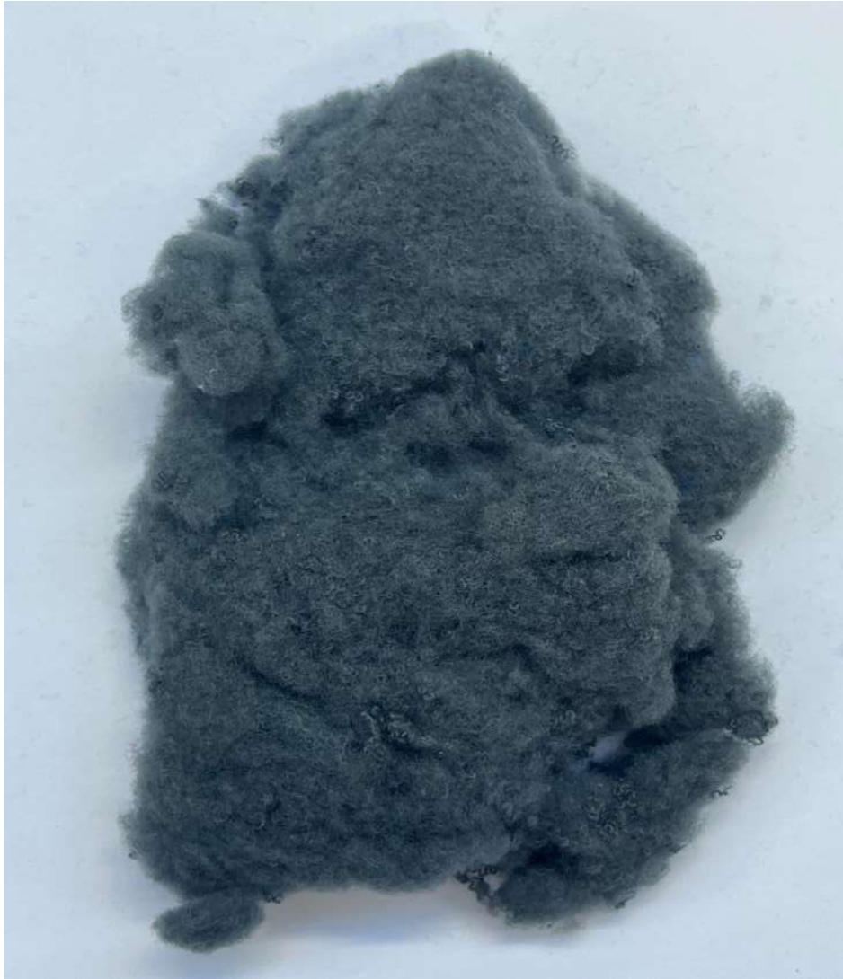
Figure C.7: picture of residue (fibers and non-opened yarns) of discolored black cotton after shredding.
