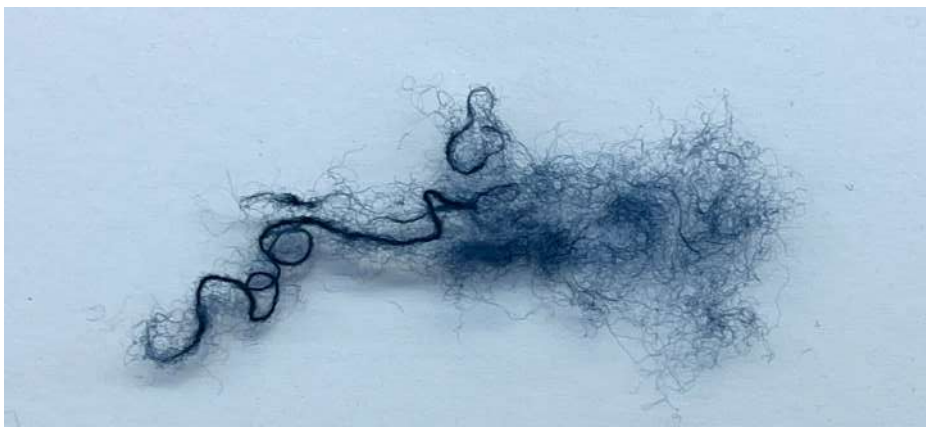
Figure C.4: detailed picture of fibers and non-opened yarns of black-dyed cotton after shredding.
