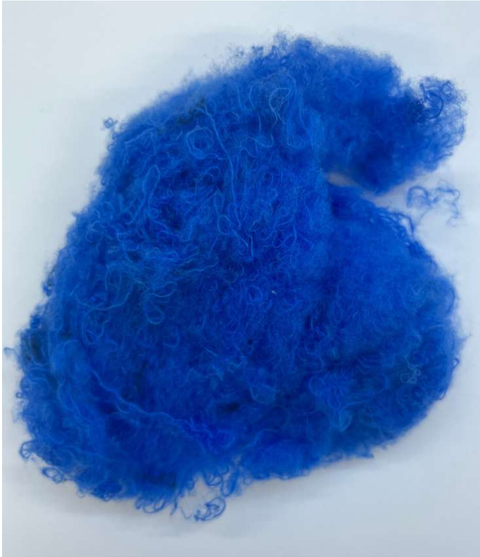
Figure C.5: picture of residue (fibers and non-opened yarns) of blue-dyed cotton after shredding.
