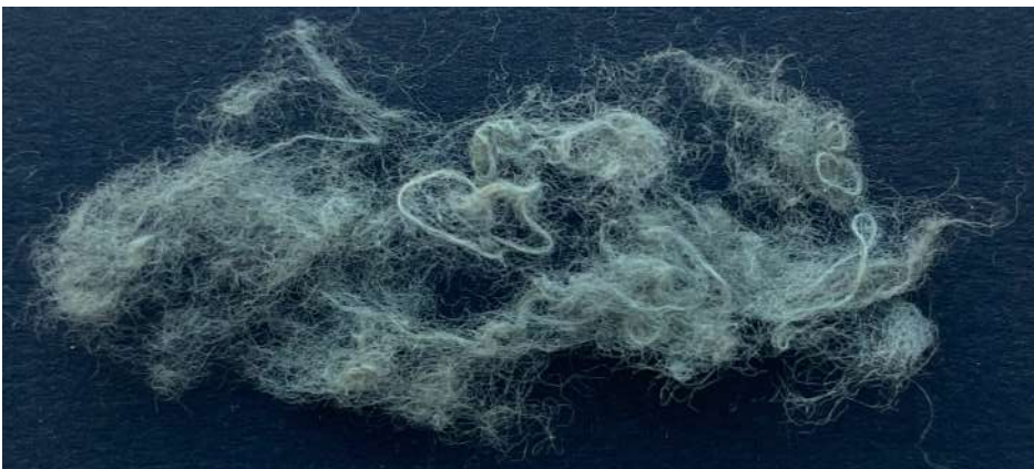
Figure C.8: detailed picture of fibers and non-opened yarns of discolored blue cotton after shredding.
