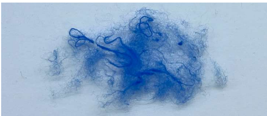
Figure C.6: detailed picture of fibers and non-opened yarns of blue-dyed cotton after shredding.
