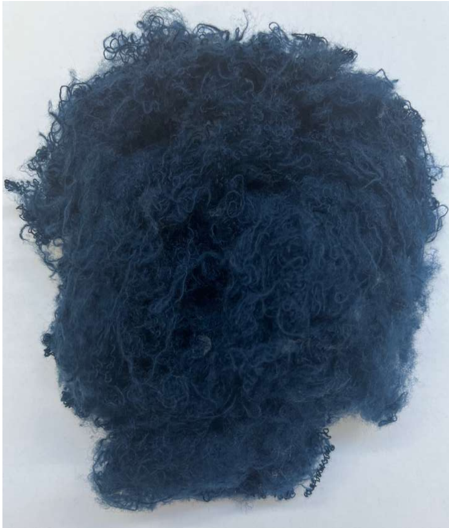
Figure C.3: picture of residue (fibers and non-opened yarns) of black-dyed cotton after shredding.
