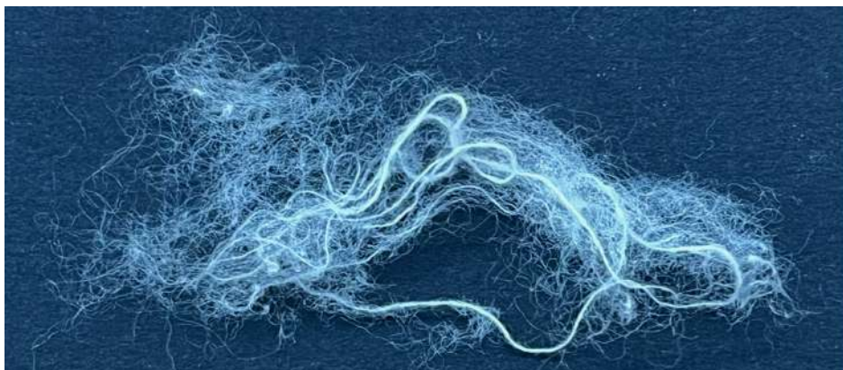
Figure C.2: detailed picture of fibers and non-opened yarns of raw cotton after shredding.
