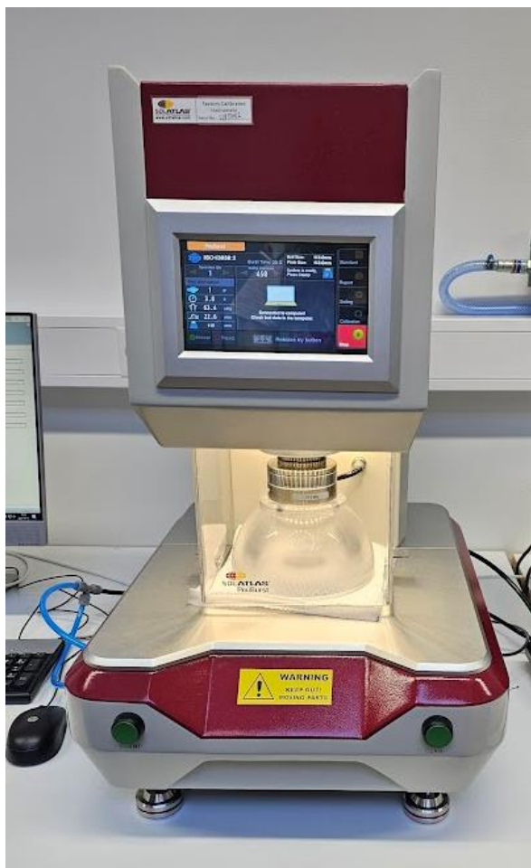
FIGURE 2, THE MACHINE USED FOR THE BURST STRENGTH TESTING WHILE IT IS BEING IN USE.
