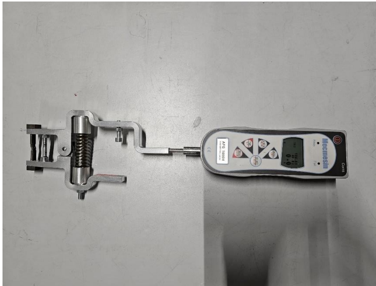
FIGURE 3, THE INSTRUMENT USED FOR THE BITE TEST WHICH CONSISTS OF A FORCE GAUGE METER AND THE DETACHABLE METAL TEETH.
