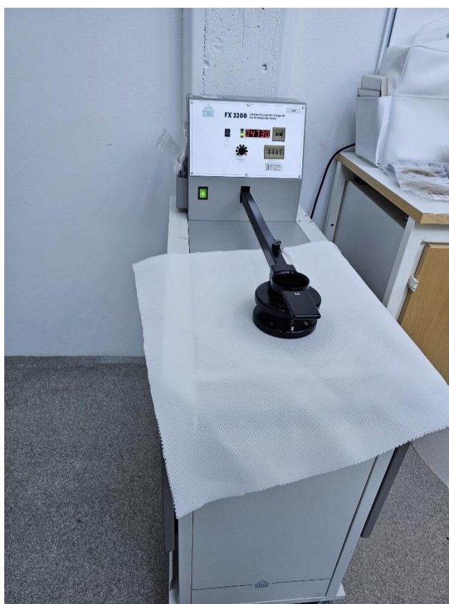
FIGURE 1, THE AIR PERMEABILITY TESTER MACHINE
