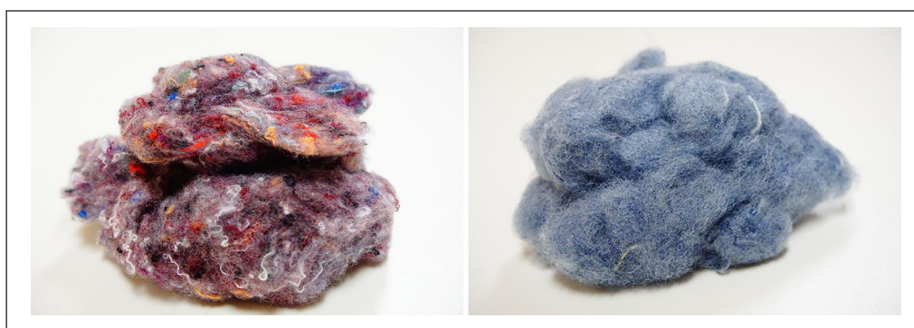
Figure 9. Barely worn fractions of torn single-jersey to the left and denim to the right.
