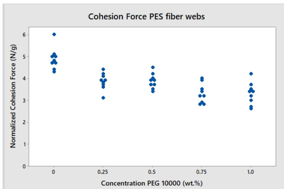
Figure 1 Tensile test result of carded webs.
