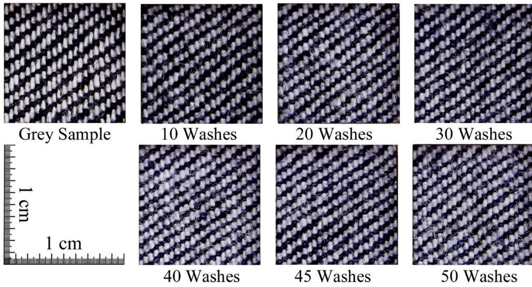
Figure 14 Microscopic images of the backside of fabric A along all washing stages to determine the yarn count per cm<sup>2</sup>.
