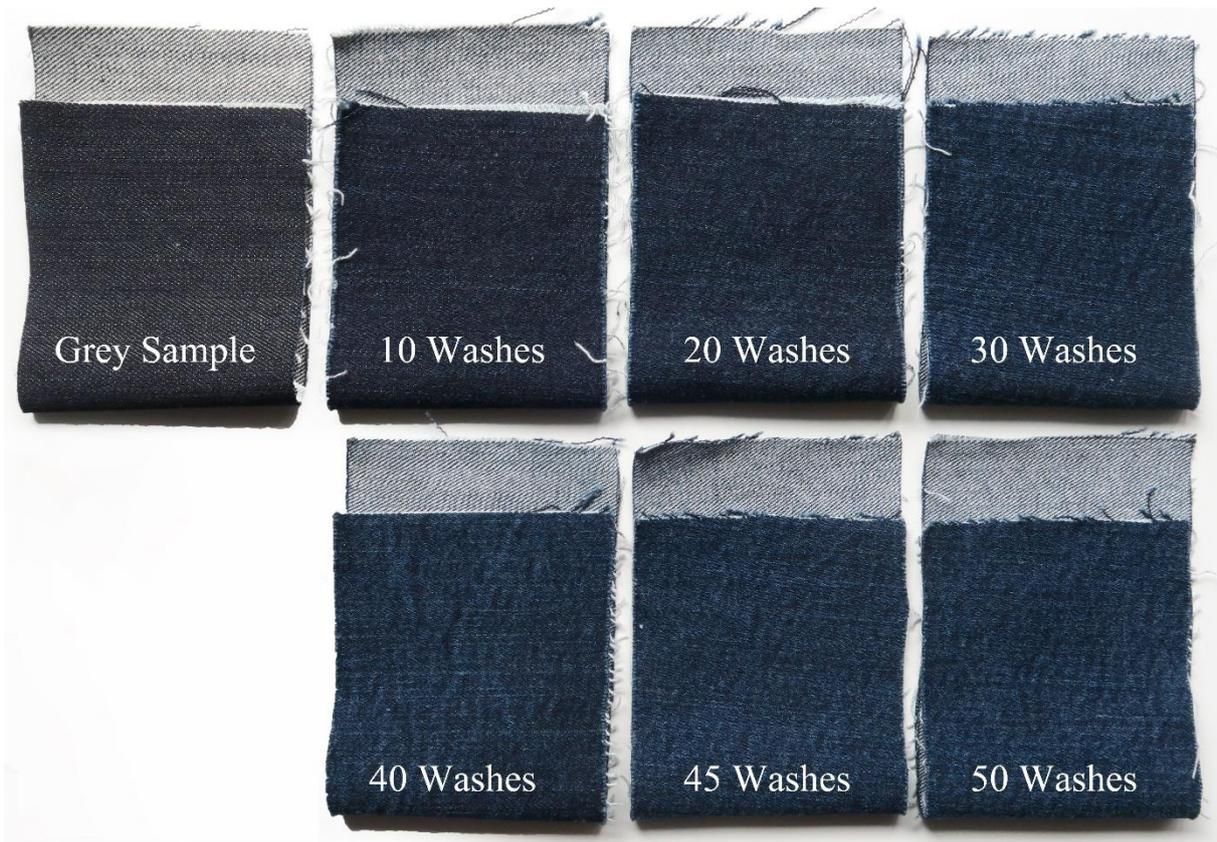
*Figure 5 Representative Samples of Fabric A for each washing and drying stage.*
