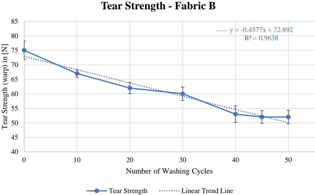
Figure 12 Visual presentation of the alteration of tear strength of fabric B in the course of washing and drying.
