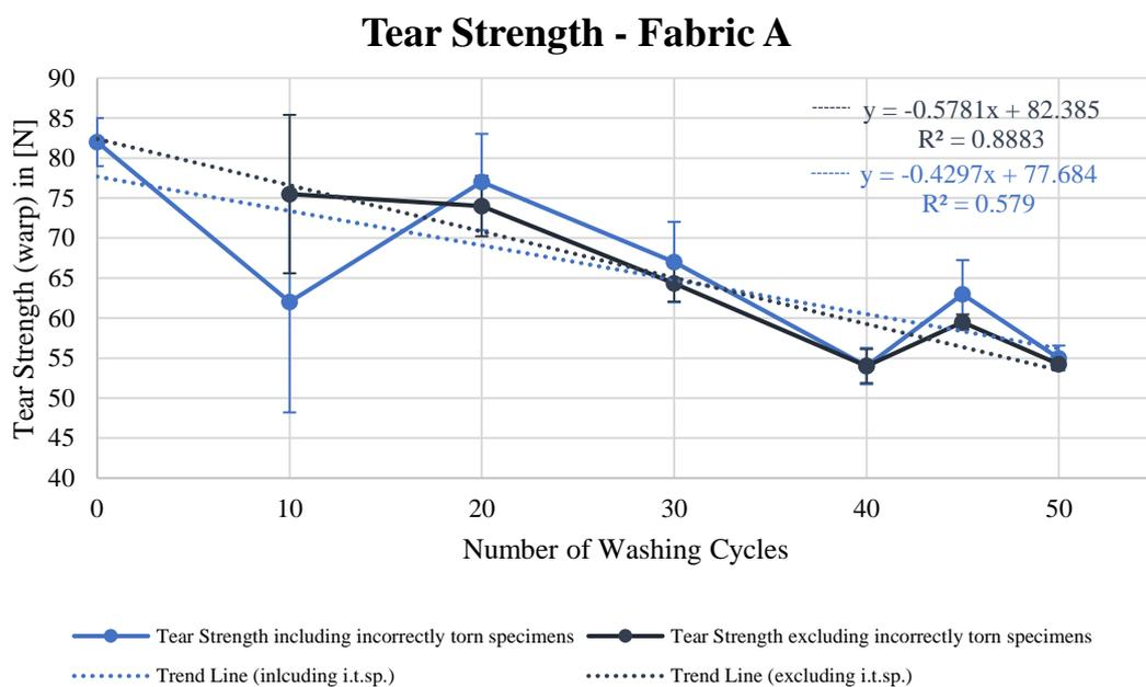
Figure 11 Visual presentation of the alteration of tear strength of fabric A in the course of washing and drying
