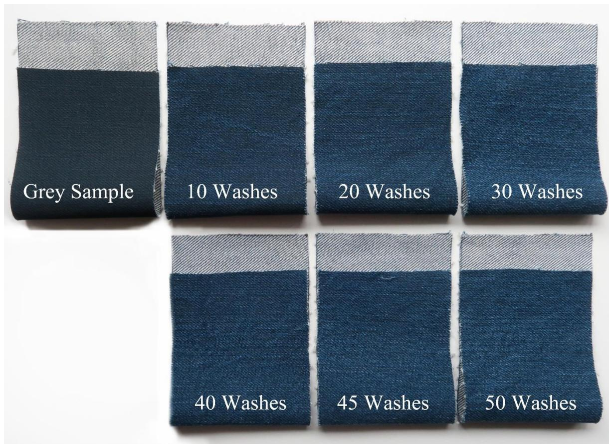
*Figure 6 Representative Samples of Fabric B for each washing and drying stage.*
