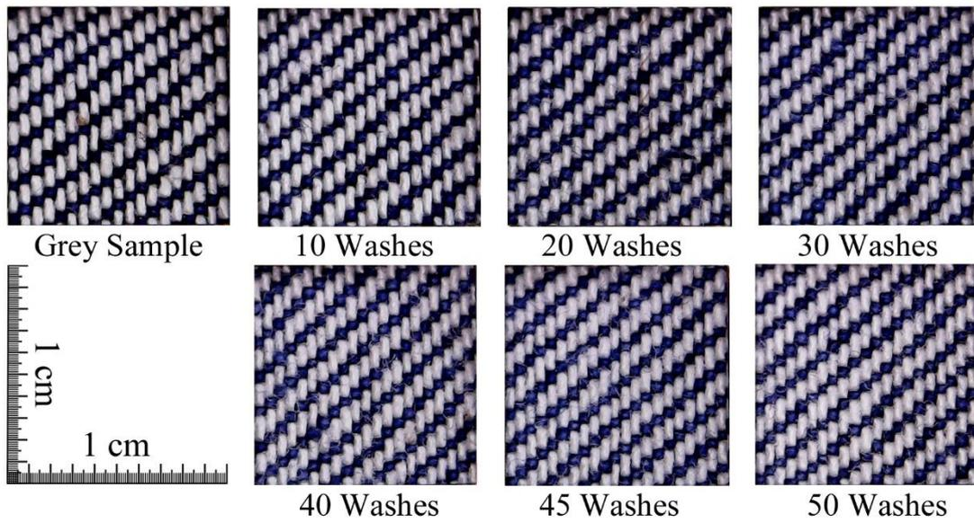
Figure 15 Microscopic images of the backside of fabric B along all washing stages to determine the yarn count per cm<sup>2</sup>.
