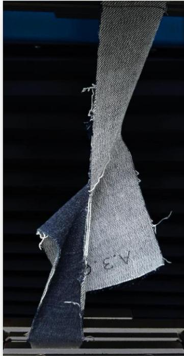
Figure 9 correctly (lengthwise) torn specimen
