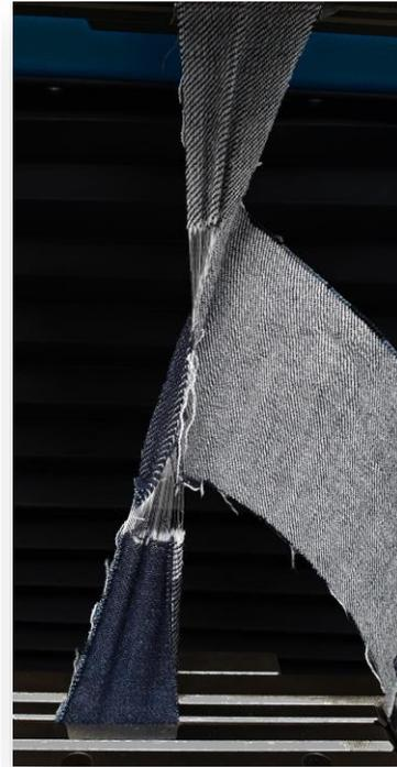
Figure 10 incorrectly (across weft) torn specimen
