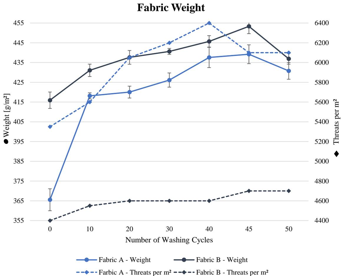
Figure 13 Visual presentment of the alteration of the fabric weight in the course of washing and drying.
