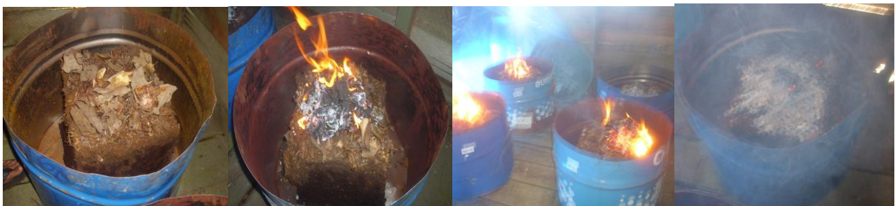
Figure 3. Peatland fire experiment: impact of water content on biomass loss
