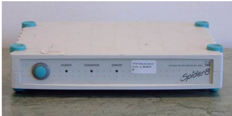
Figure 2. Spider 8, a strain gage measurement device.
