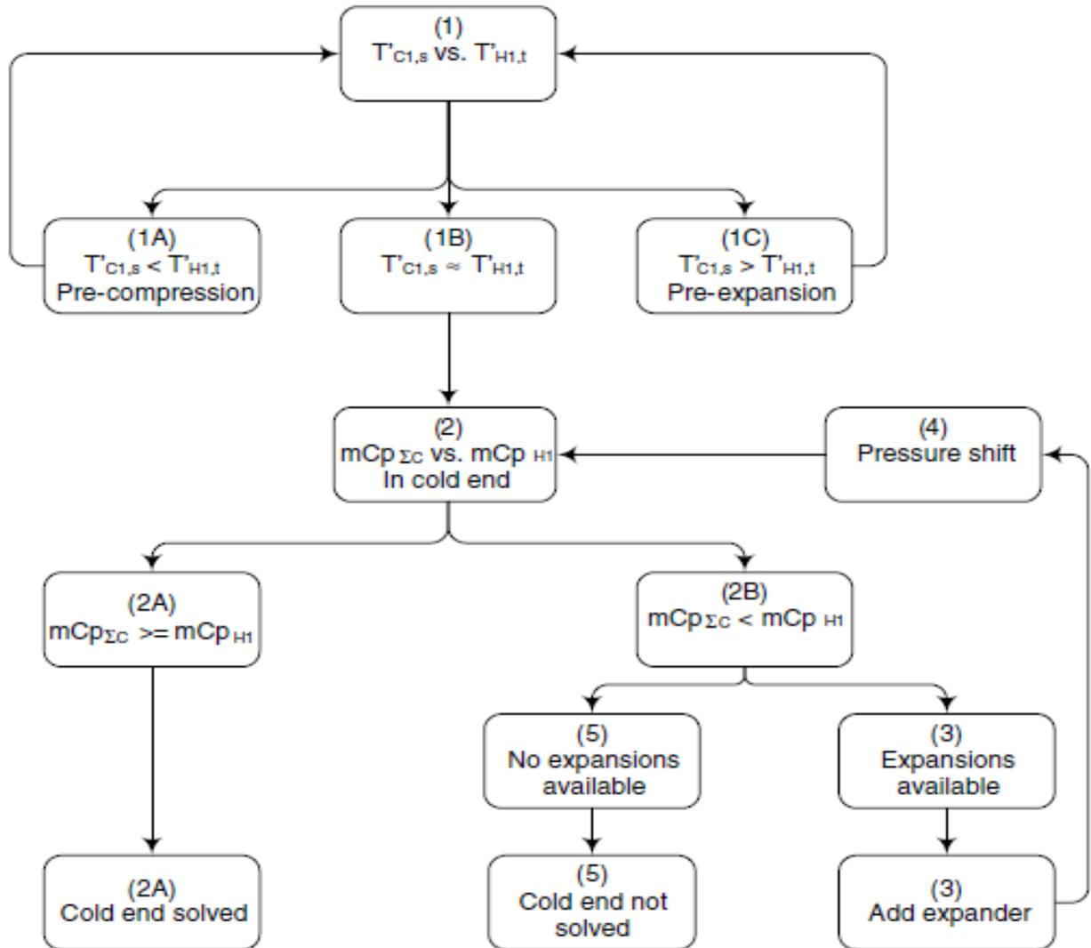
**Fig – 12.** Procedure for cooling a hot stream by utilizing pressure based exergy in a cold stream. (Aspelund et al., 2007)
