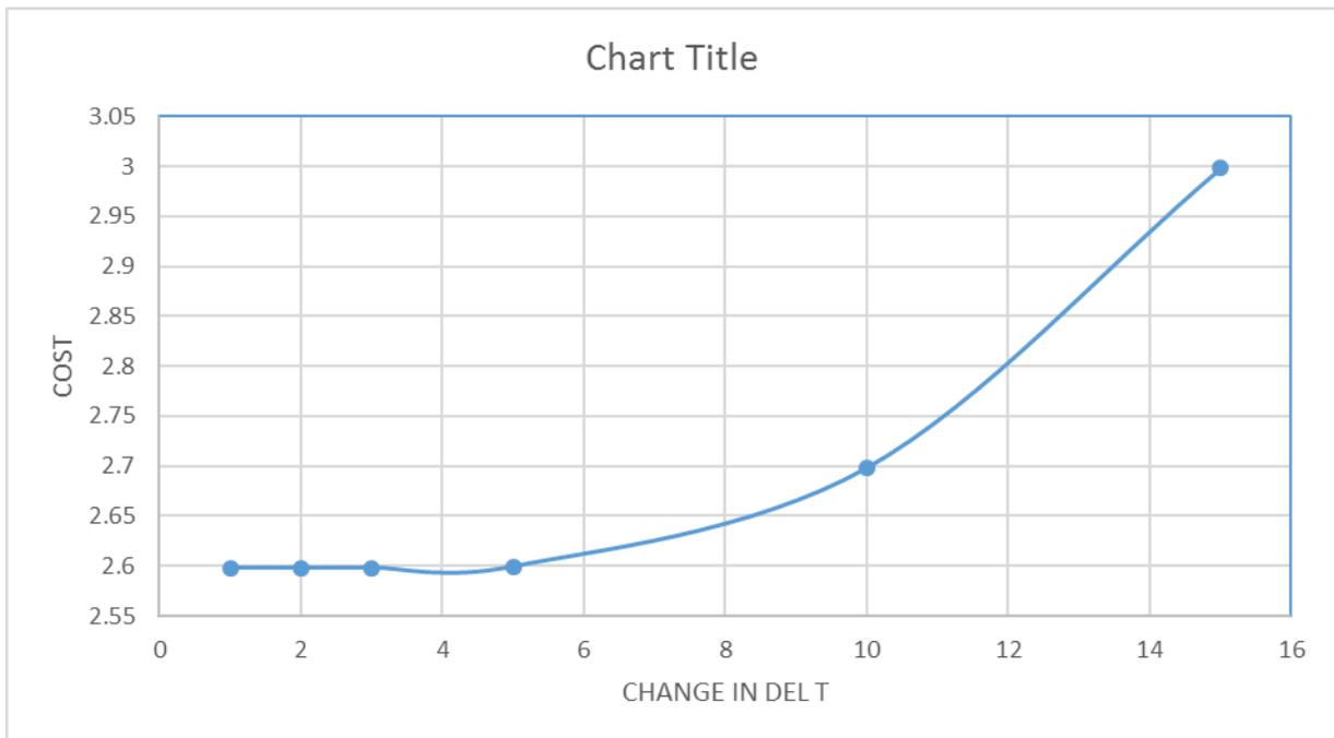
**Fig – 18.** A graph plotted between the  $\Delta T_{\min}$  and the capital cost.
