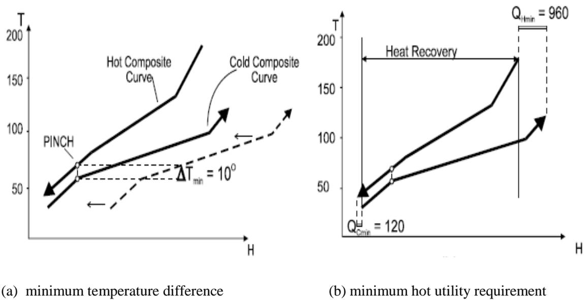
**Fig – 4.** Combined composite curve to determine energy targets (March, 1998)
