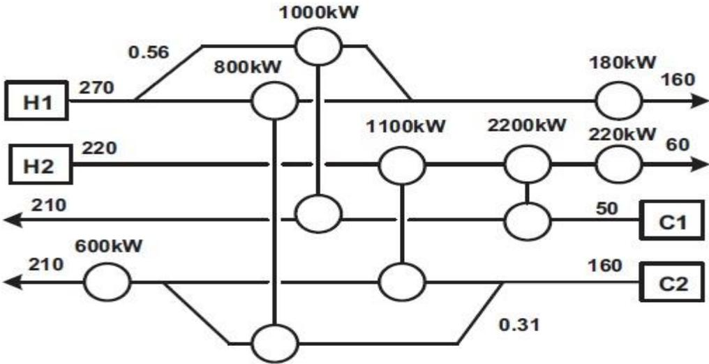
(a) Actual placement of heat exchangers from reference model. (Escobar and Trierweiler, 2013)
