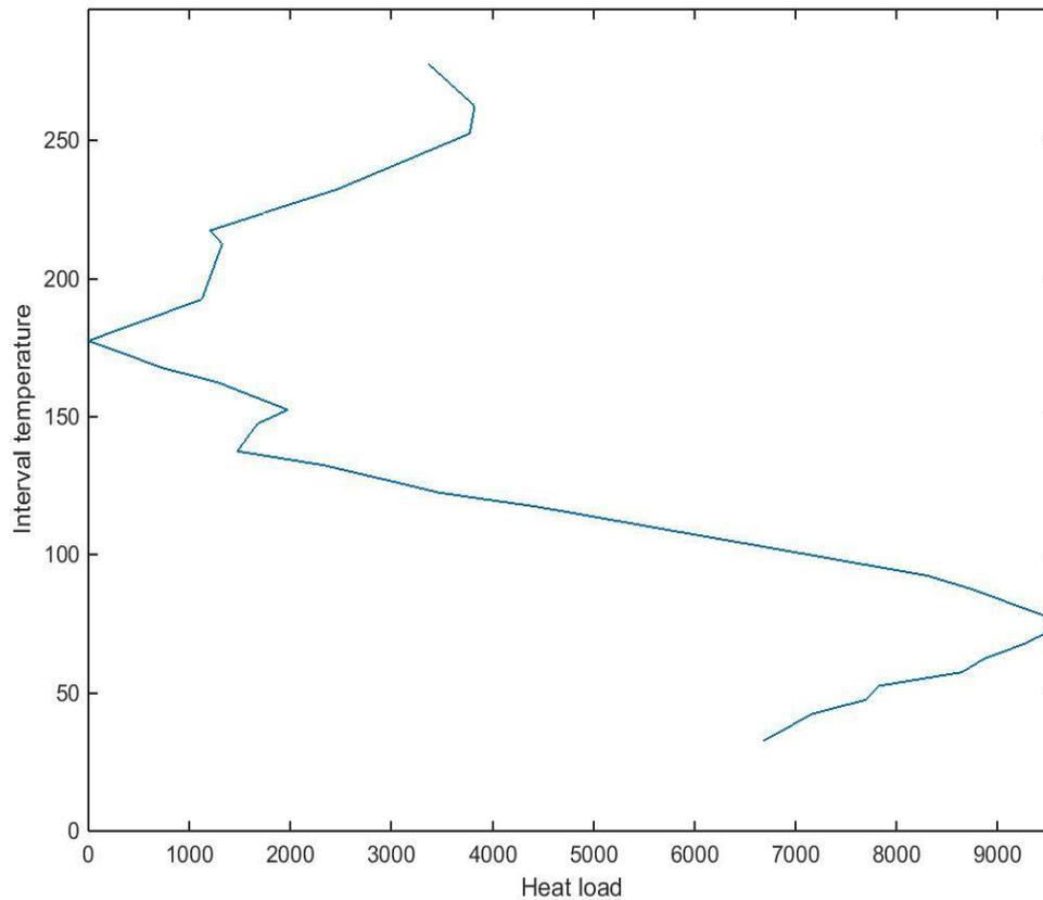
**Fig – 20.** Grand composite curve from above data.
