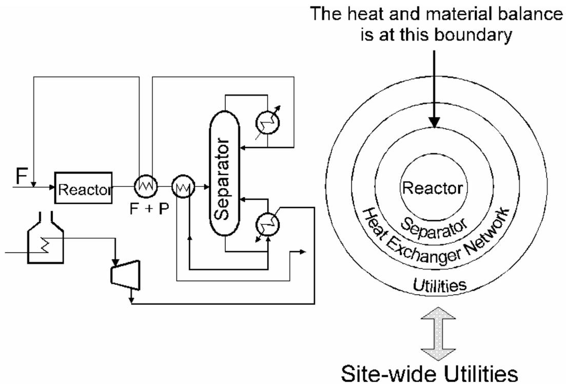
Fig – 1. 'Onion diagram' hierarchy in process design (March, 1998)
