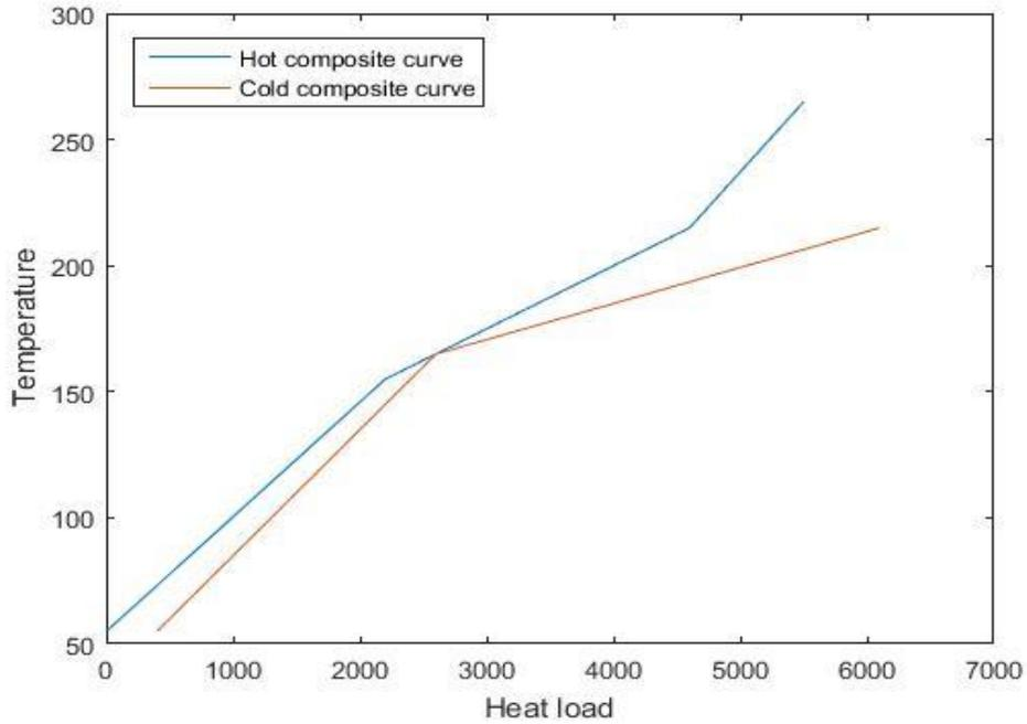
(a) Hot and cold composite curve obtained from MATLAB for the above data.
