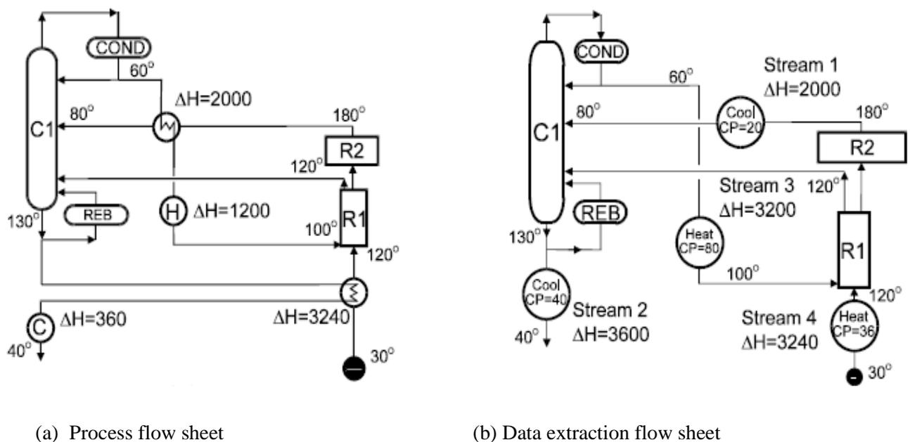
**Fig – 2.** Data extraction for Pinch Analysis.(March, 1998)
