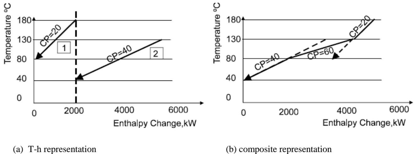
**Fig – 3.** Construction of two hot composite curves (March, 1998)
