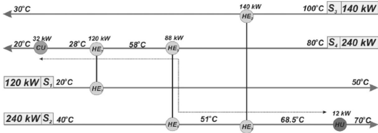
**Fig – 10.** Heat exchanger network after using of rule for loops through the pinch point. (Anastasovski, 2014)
