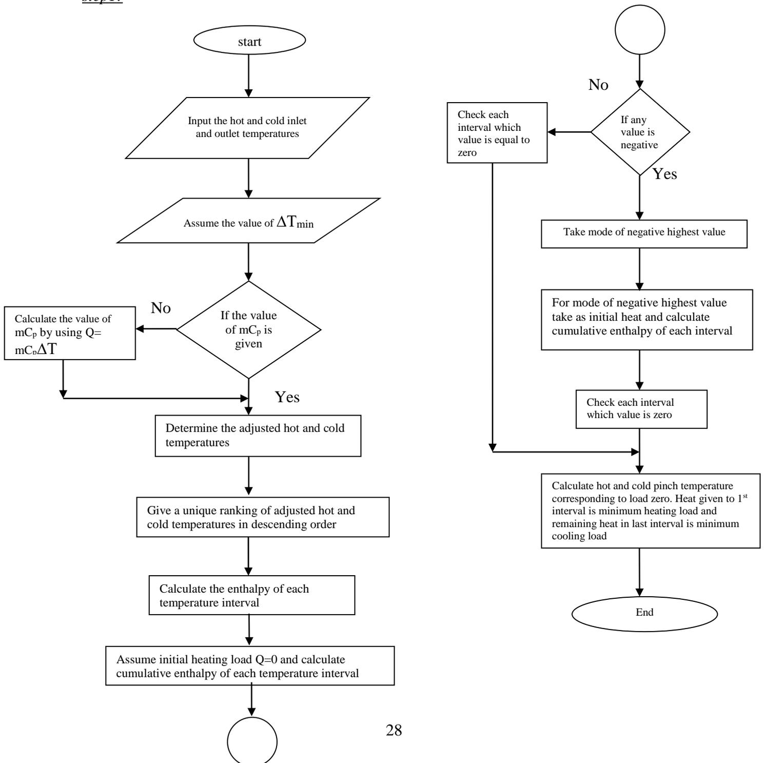
The above flow chart explains the steps in Pinch Analysis (Tewari et al., 2015). In the Pinch Analysis step, the actual steam temperatures are converted to interval temperatures using the below equations,
