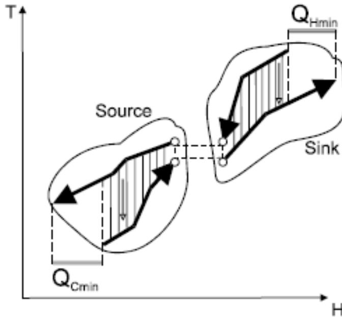
**Fig – 5.** The pinch divides the problem into source and sink (March, 1998)
