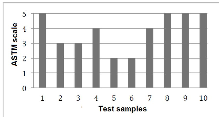
**Figure 1.** Pilling effect on the test samples after 7000 turns due to the ASTM D3512 scale.
