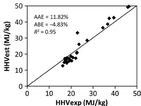
**Figure 4.** Comparison between the experimental and the estimated HHV by Dulong's correlation.
