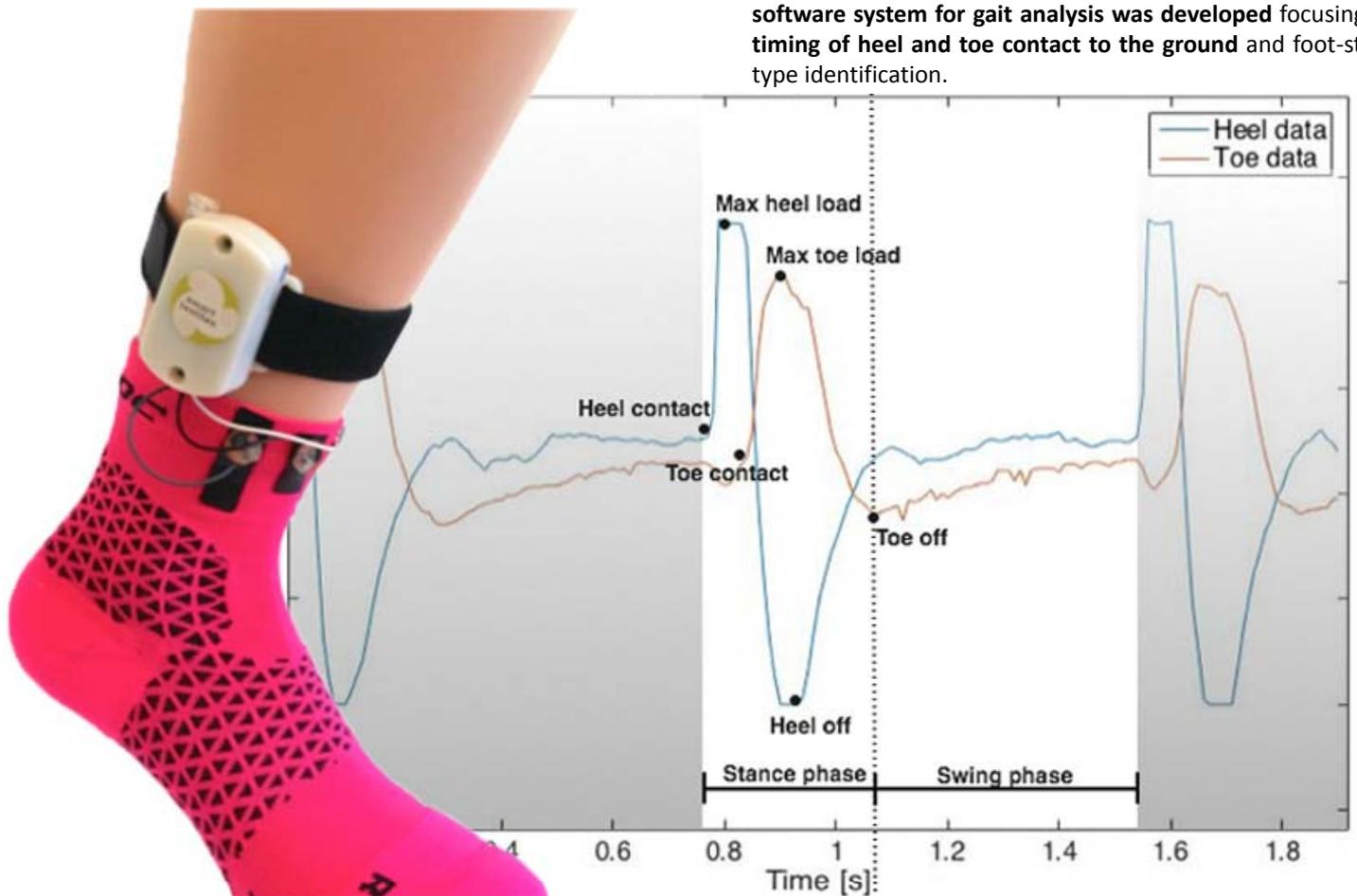
Figure 1. Illustration of the complete system. The sock is instrumented with piezoelectric fibers in heel and toe and connected to a Bluetooth unit sending to a smartphone. The graph shows a short sequence of the signals collected during a run. Distinct events of the step cycle is identified (marked) defining the step profile. Step profiles are then isolated and analyzed separately in order to be classified as either heel-, mid- or toe-strike.
